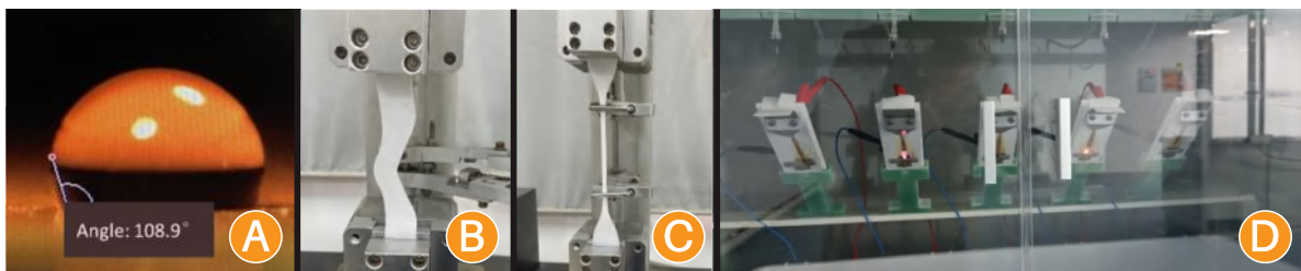
(A) Static contact angle (C) Tensile strength test
