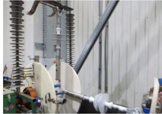
Tracking and Erosion Test (wheel method) of suspension insulator
