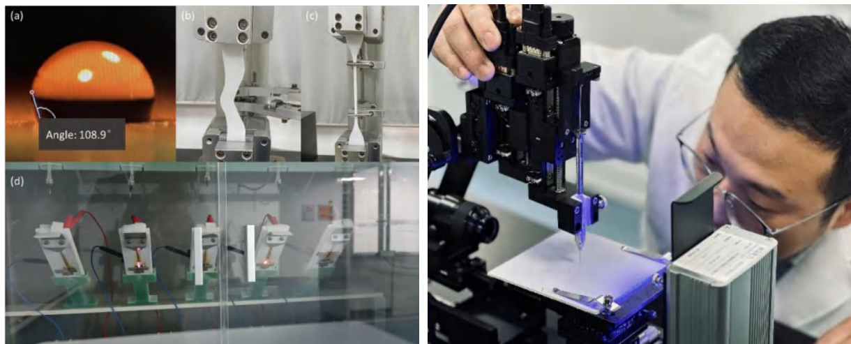
Testing: (a) Static contact angle (b) Tearing strength test (c) Tensile strength test (d) Tracking and erosion resistance test
