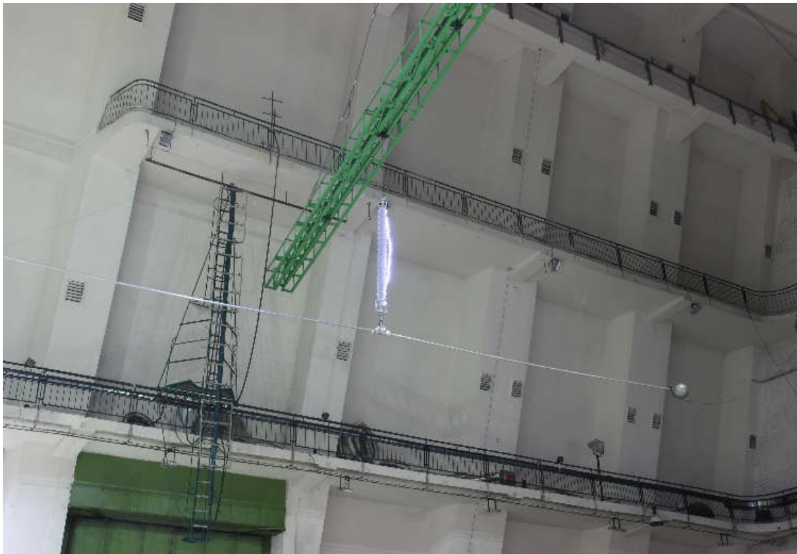
Figure 4 Test arrangement and flashover under the critical impulse flashover test
