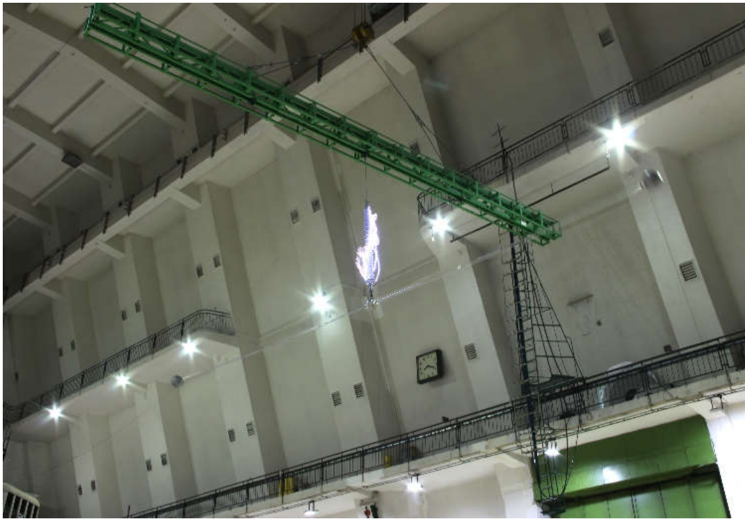
Figure 6 Test arrangement and flashover under the low-frequency dry flashover test
