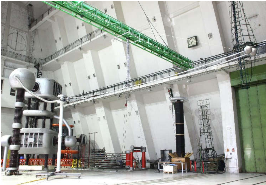
Figure 2 Test arrangement for RIV and corona tests
