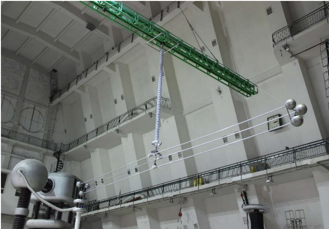
Figure 2 Test arrangement for RIV and corona tests
