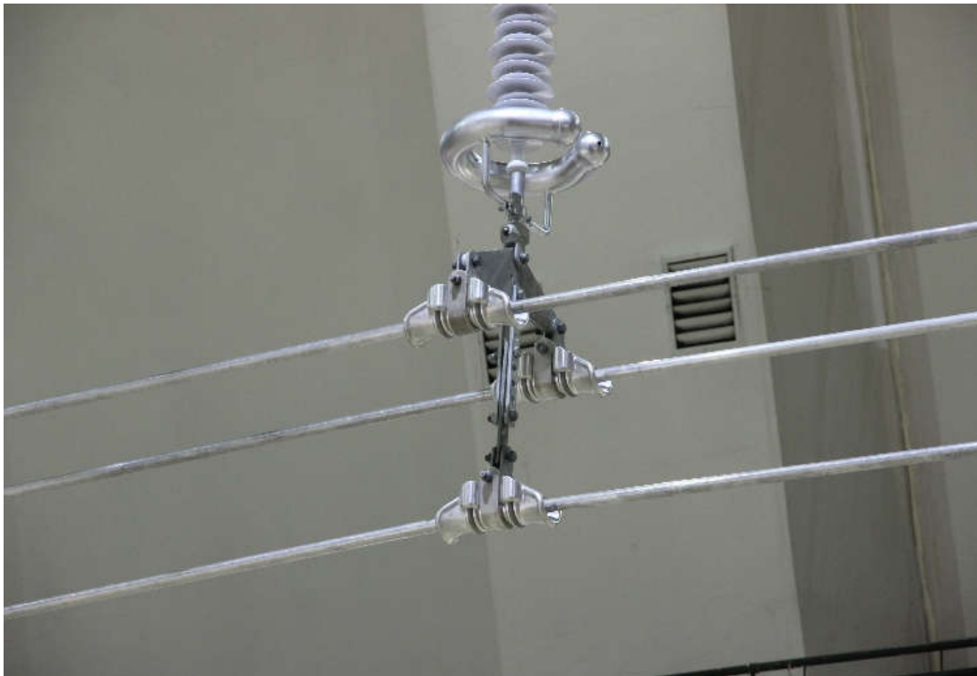
Figure 3 Test arrangement for RIV and corona tests
