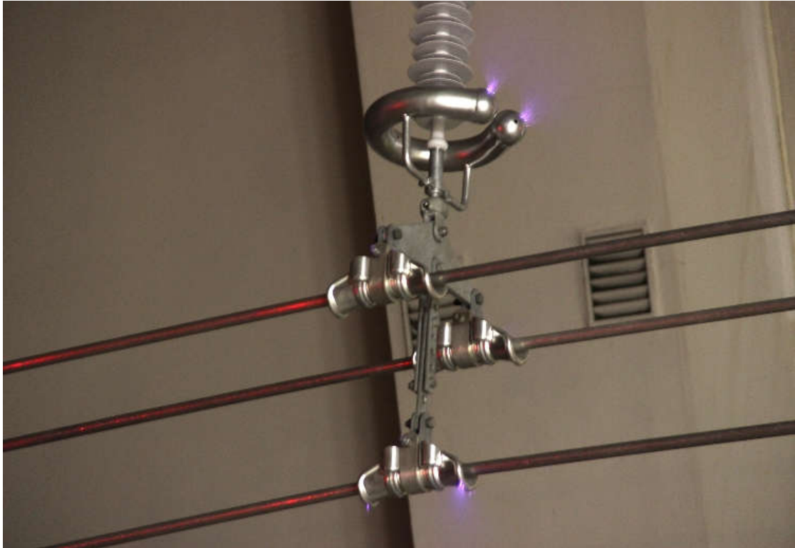
Figure 5 Test object at the test voltage of 463 kV
