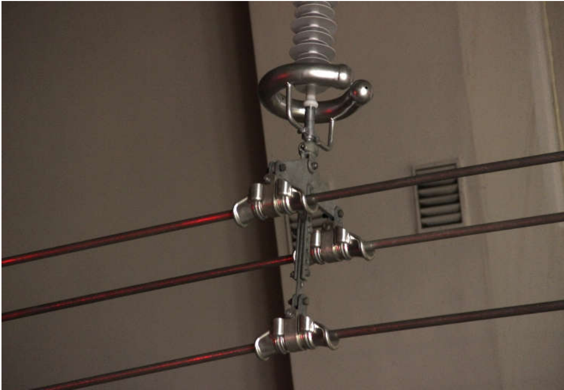
Figure 4 Test object at the test voltage of 381 kV – no positive corona
