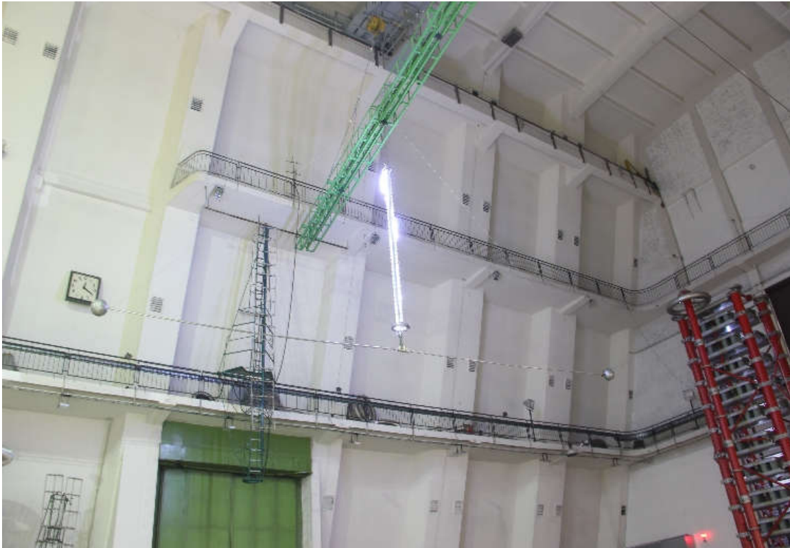
Figure 6 Test arrangement and flashover under the critical impulse flashover test
