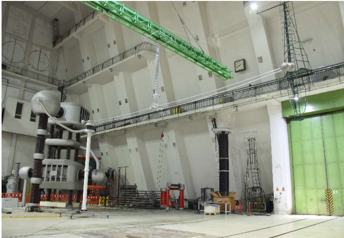
Figure 2 Test arrangement for RIV and corona tests
