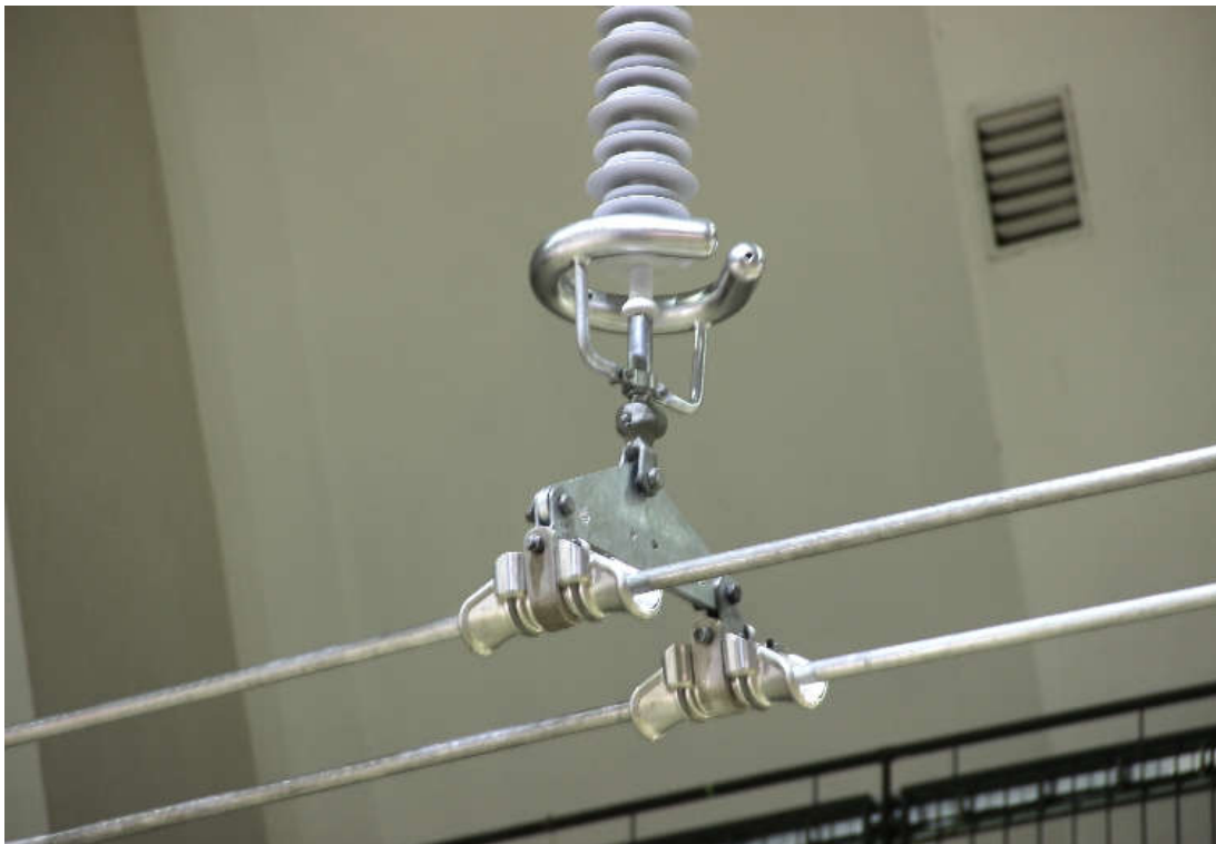
Figure 3 Test arrangement for RIV and corona tests
