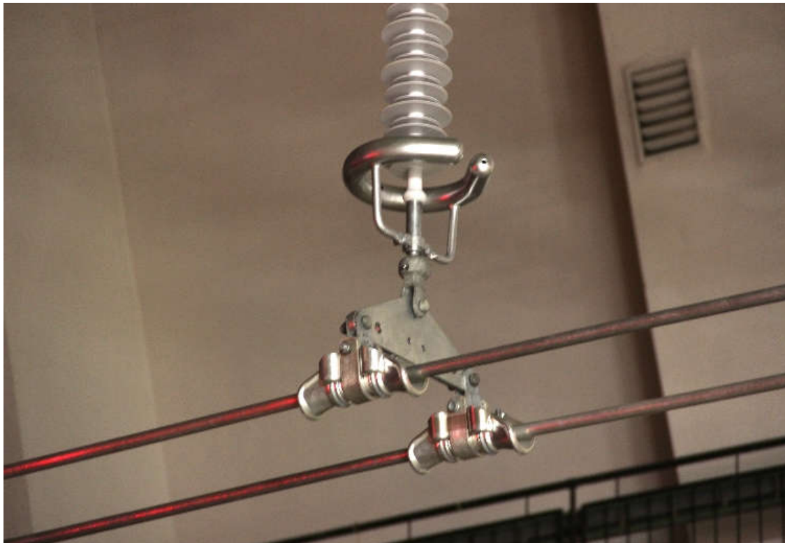
Figure 4 Test object at the test voltage of 251 kV – no positive corona
