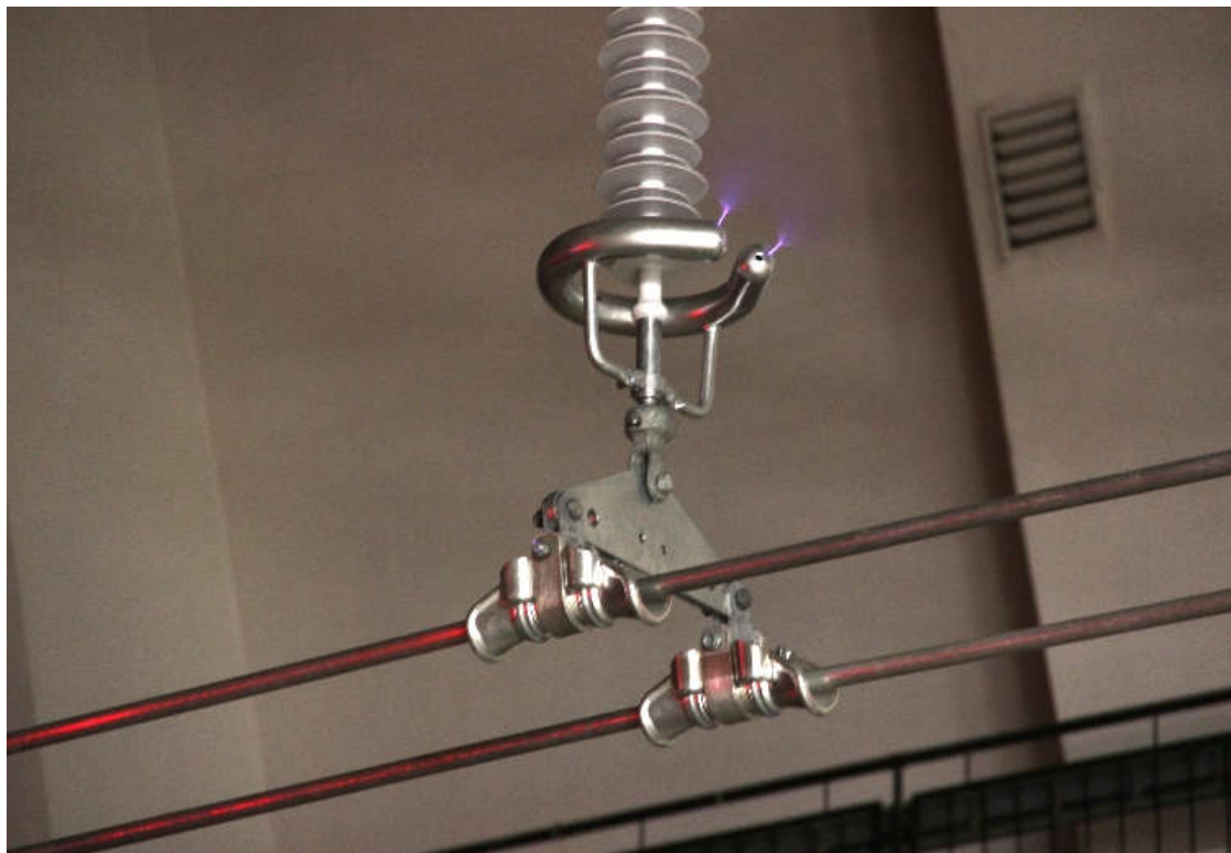
Figure 5 Test object at the test voltage of 326 kV
