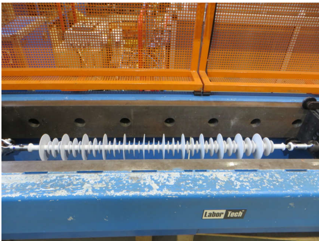
Figure 16 Mechanical failing load test, test sample No. 7
