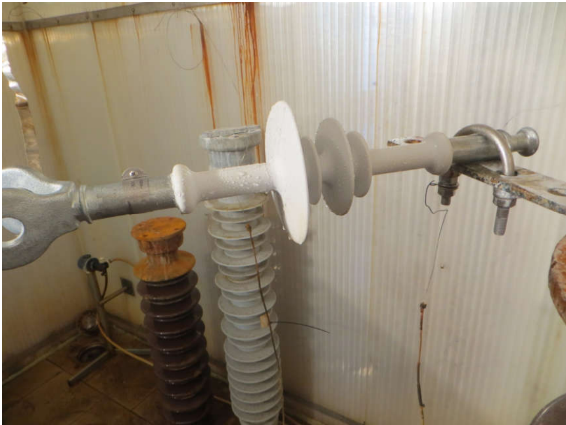
Figure 4 Test sample in horizontal test position, before housing tracking and erosion test
