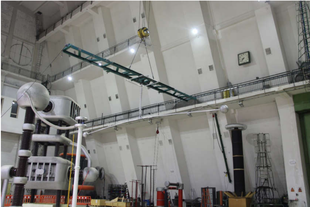
Figure 3 Test arrangement under the radio – influence voltage test
