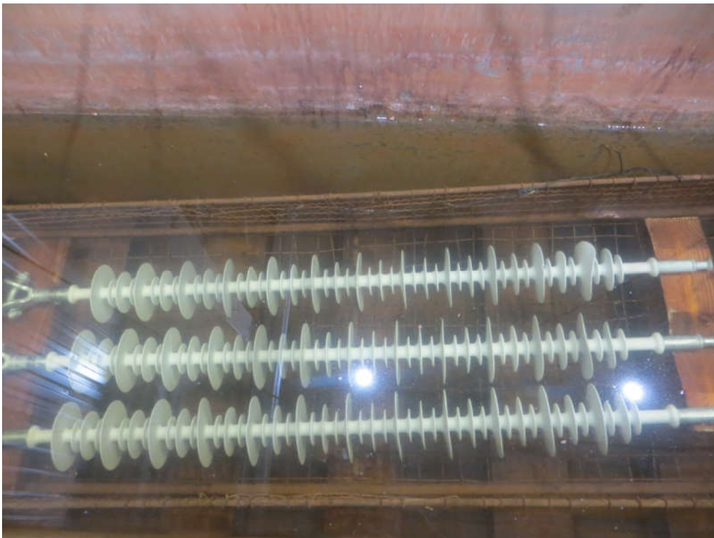
Figure 12 Test samples during water penetration test
