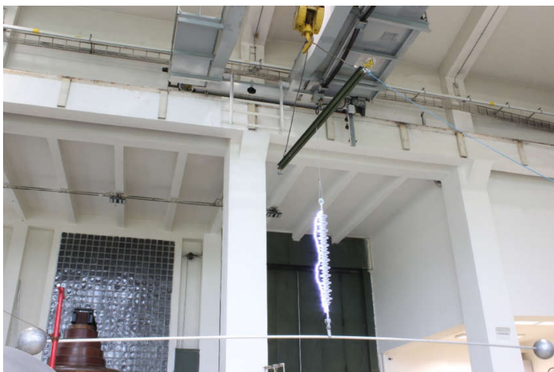
Figure 6 Test arrangement and flashover under the low-frequency dry flashover test
