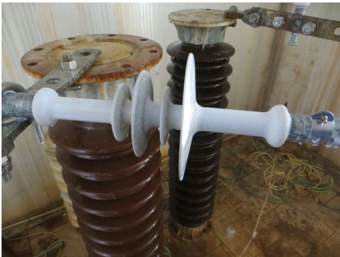
Figure 5 Test sample in horizontal test position, after housing tracking and erosion test
