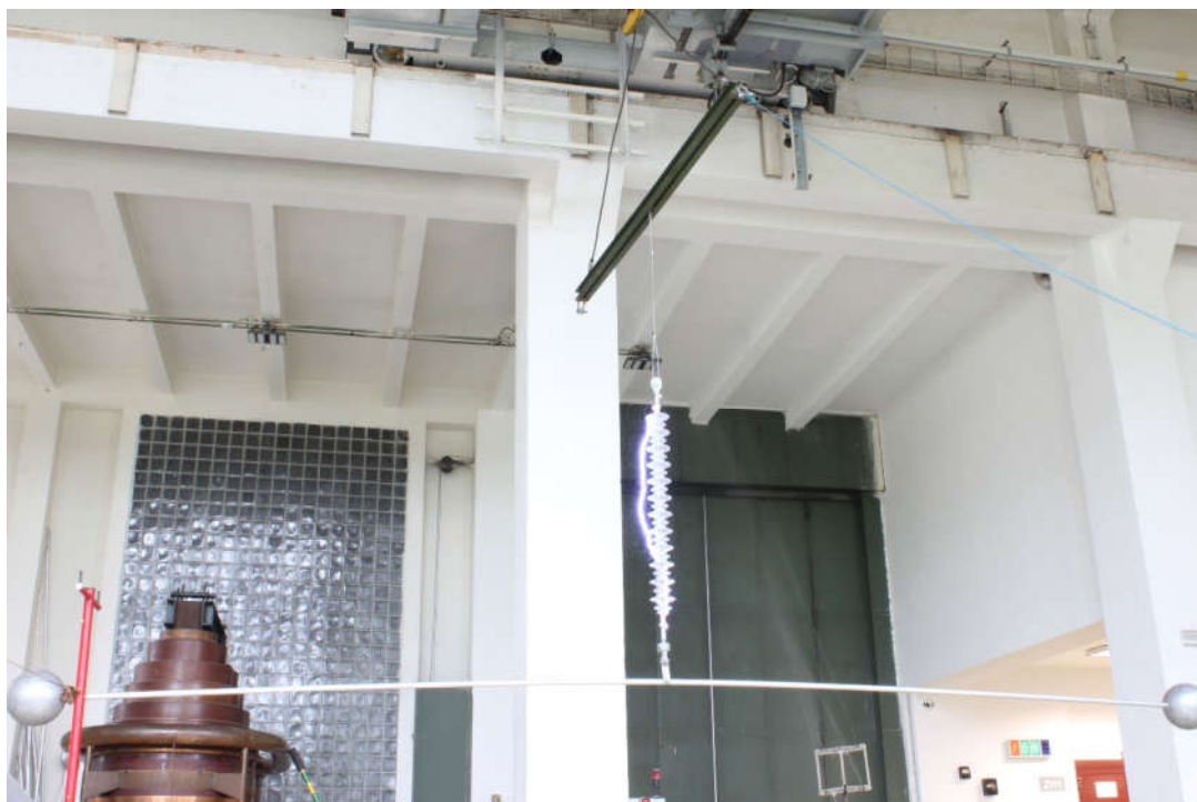
Figure 5 Test arrangement and flashover under the low-frequency wet flashover test
