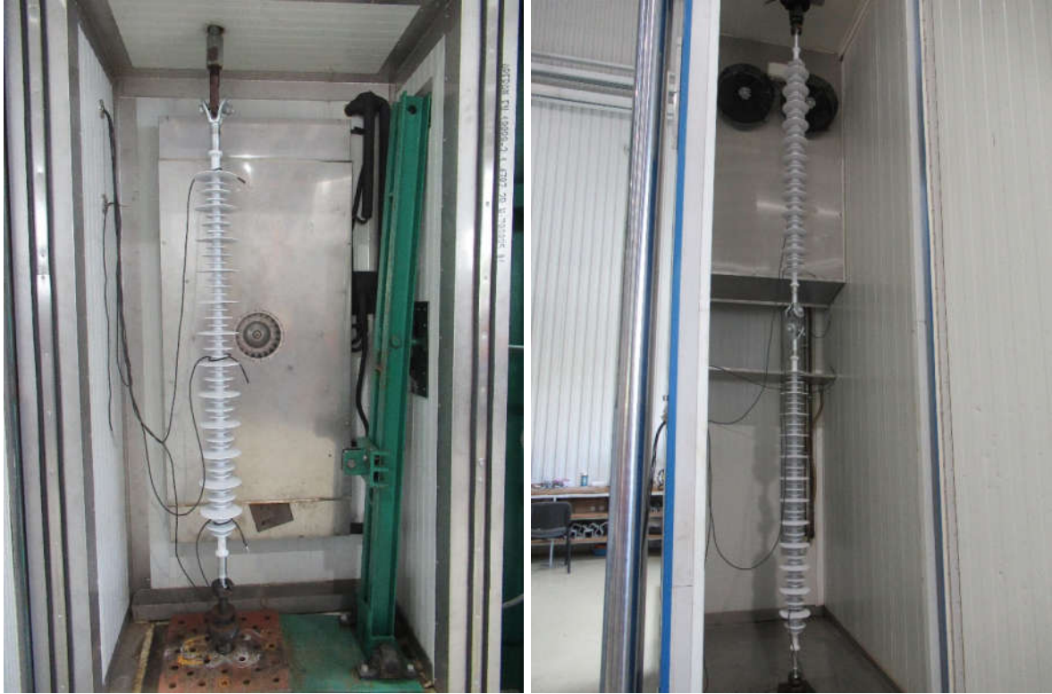
Figure 11 Test samples during thermal mechanical test
