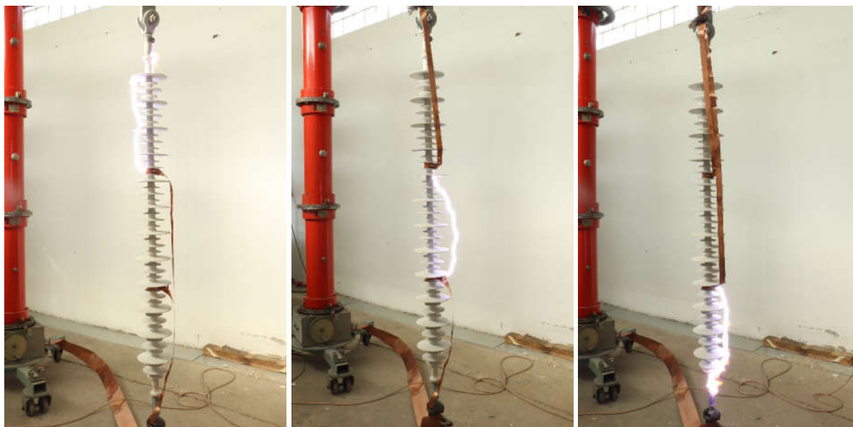
Figure 13 Test sample during the linearly rising front chopped impulse voltage test
