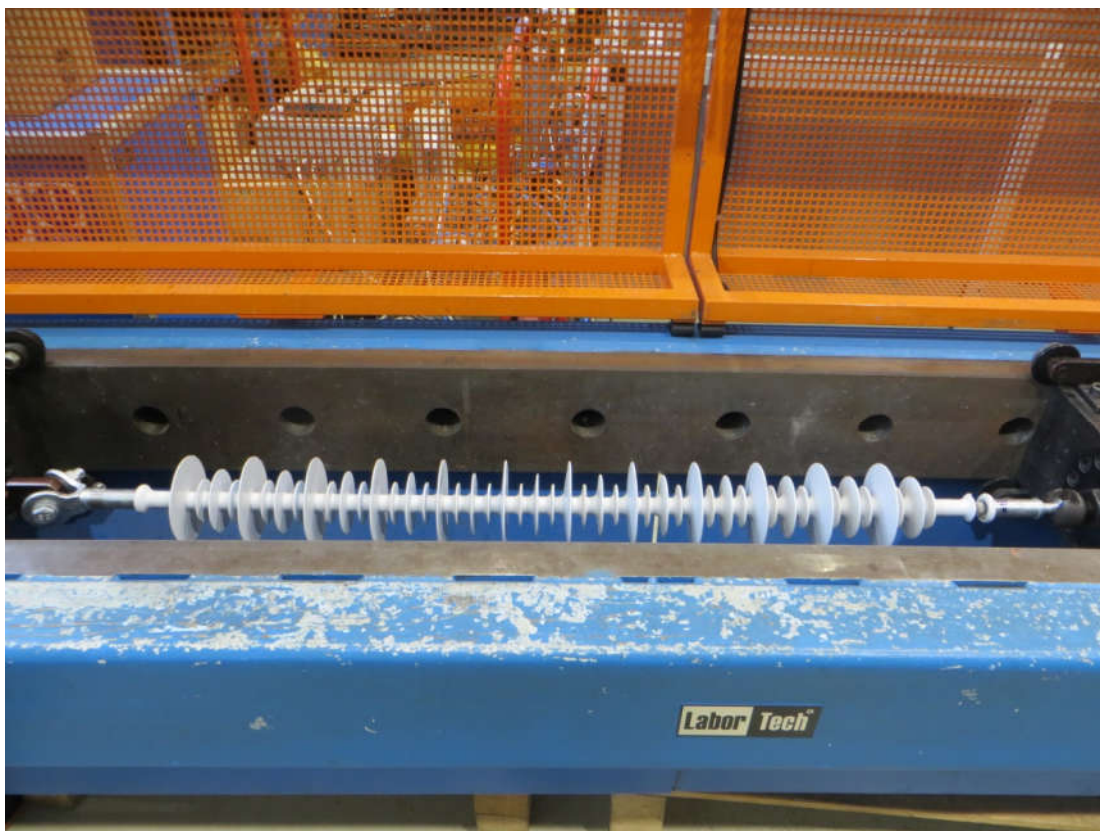
Figure 17 Mechanical failing load test, test sample No. 8
