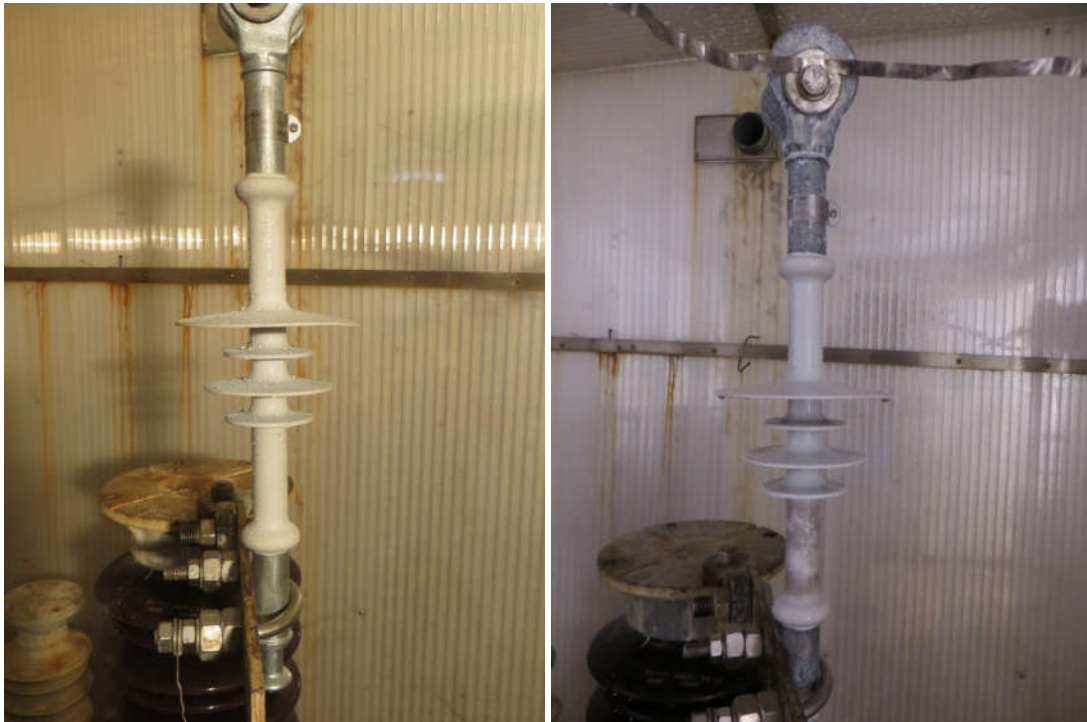
Figure 3 Test sample in vertical test position, before and after housing tracking and erosion test
