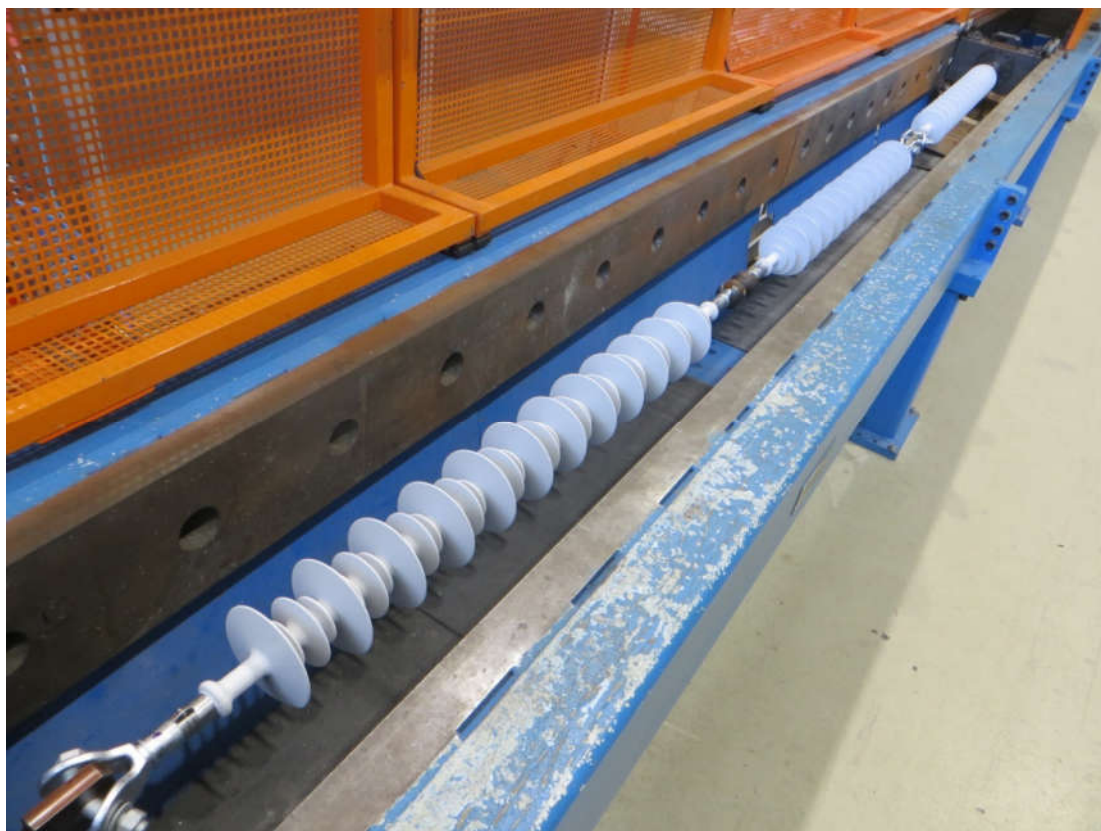
Figure 19 Withstand tensile load test, test samples No. 9, 10 and 11
