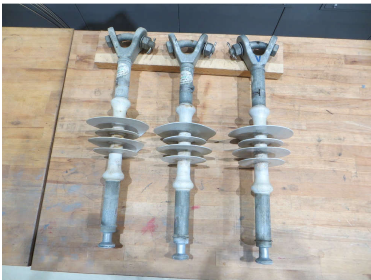
Figure 9 Composite insulator 133 kV, SML 222 kN, test samples No. 1, 2 and 3, after tracking end erosion test
