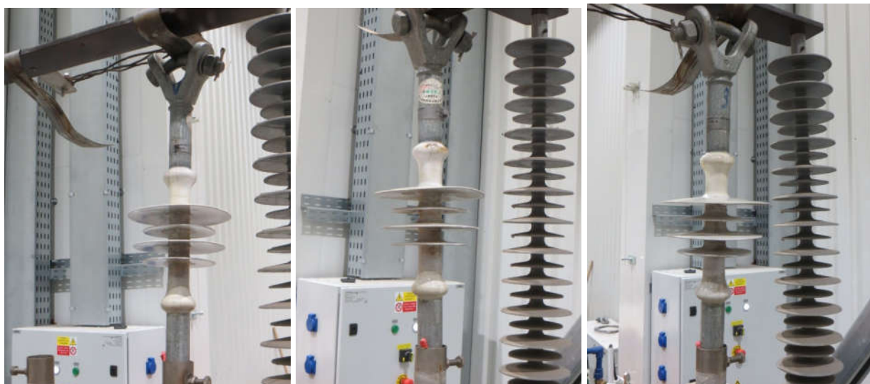
Figure 8 Composite insulator 133 kV, SML 222 kN, test samples No. 1, 2 and 3, after tracking end erosion test
