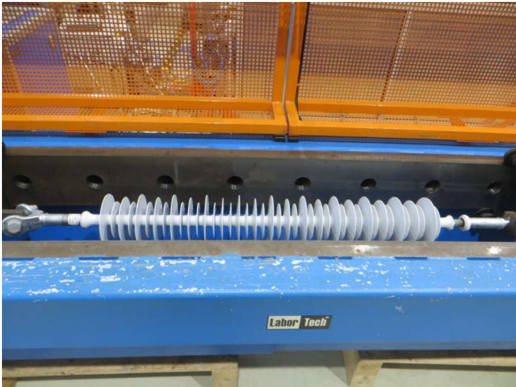
Figure 16 Test sample No. 1, after the mechanical failing load test, assembled core load-time test
