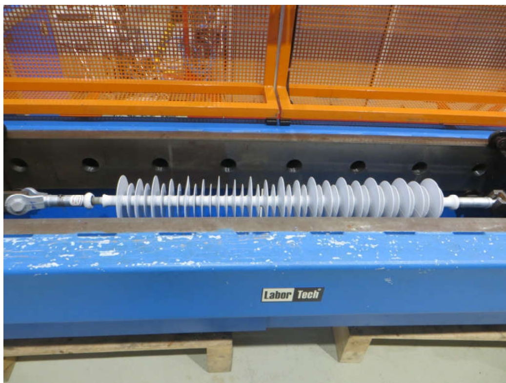
Figure 24 Test sample No. 1 after the mechanical failing load test, mechanical load-time test
