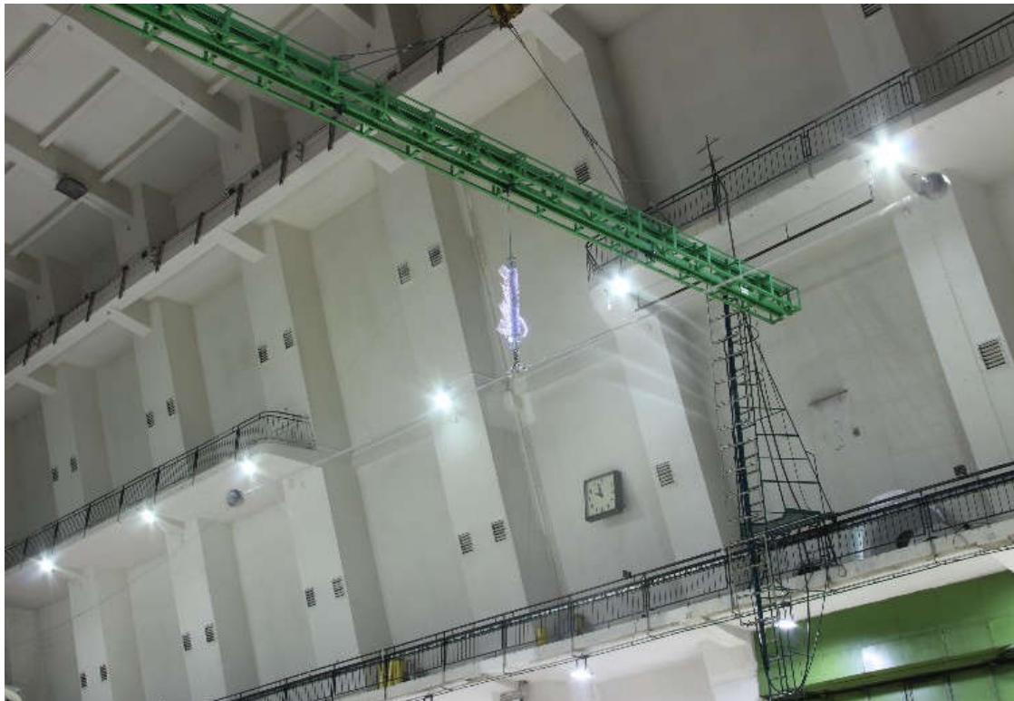
Figure 7 Test arrangement and flashover under the wet power frequency voltage flashover test
