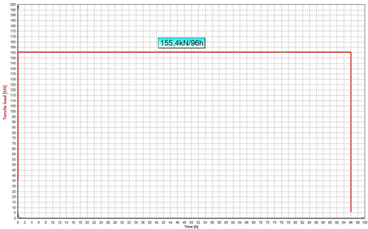
Graph 13 Record of 96 hours mechanical loading test, mechanical load-time test, test samples No. 1, 2 and 3
