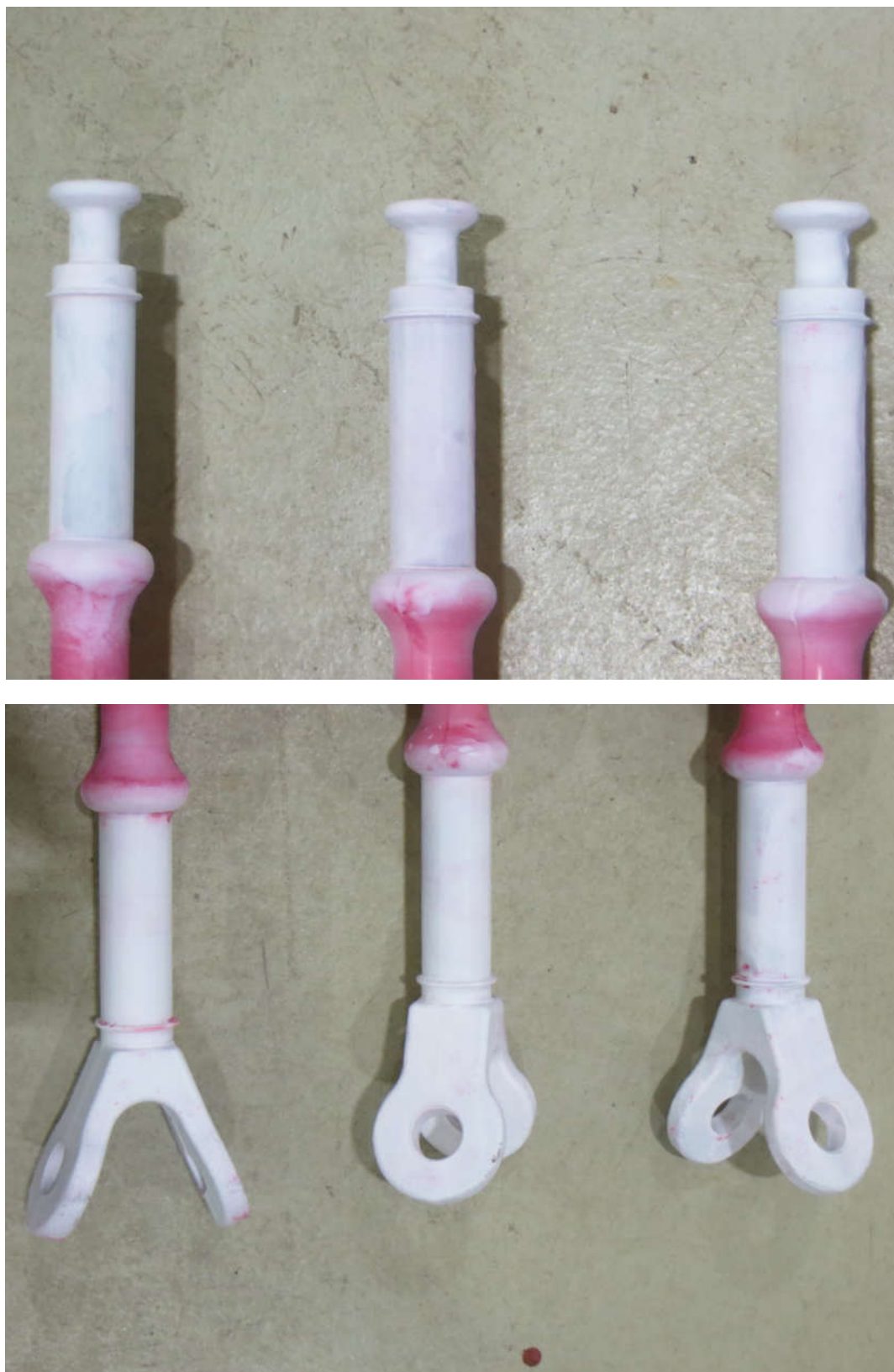
Figure 15 Test samples No. 1, 2 and 3 after diagnostic testing of the fittings, thermal-mechanical test
