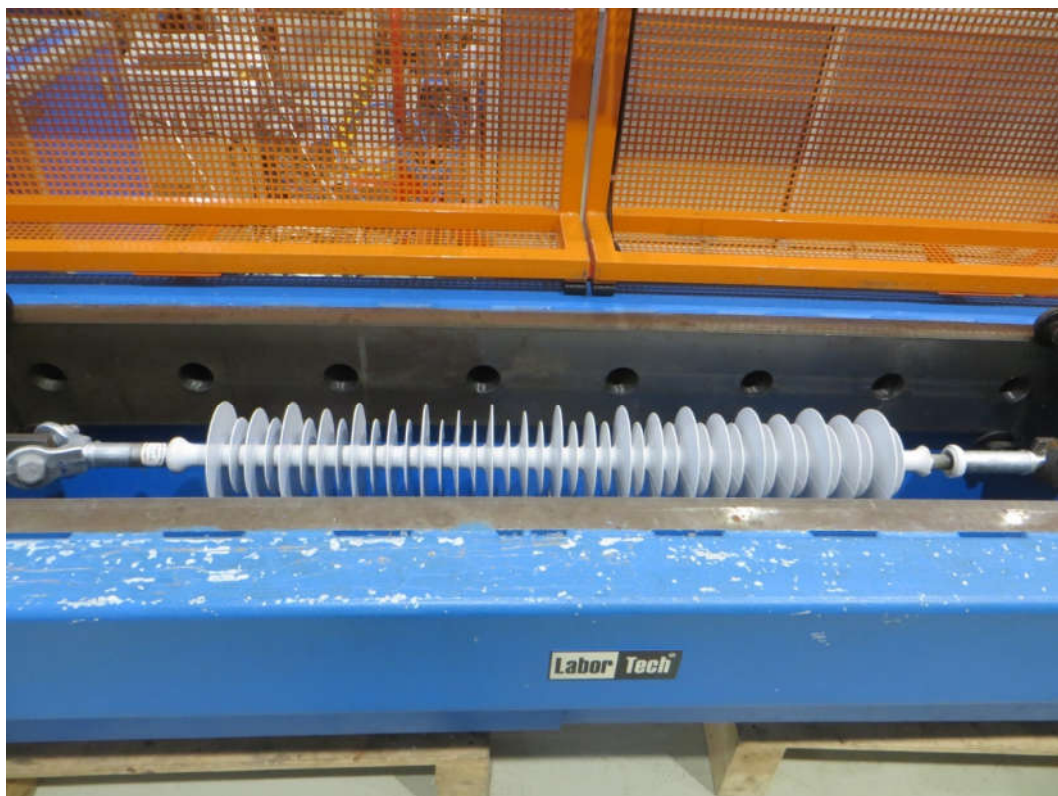
Figure 10 Test sample No. 1, after the mechanical failing load test
