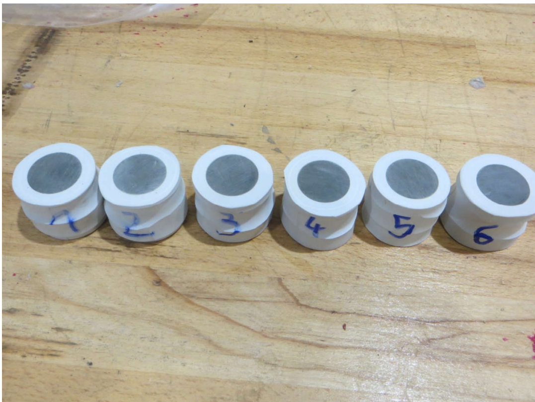
Figure 17 Test specimens after the voltage test – water diffusion test
