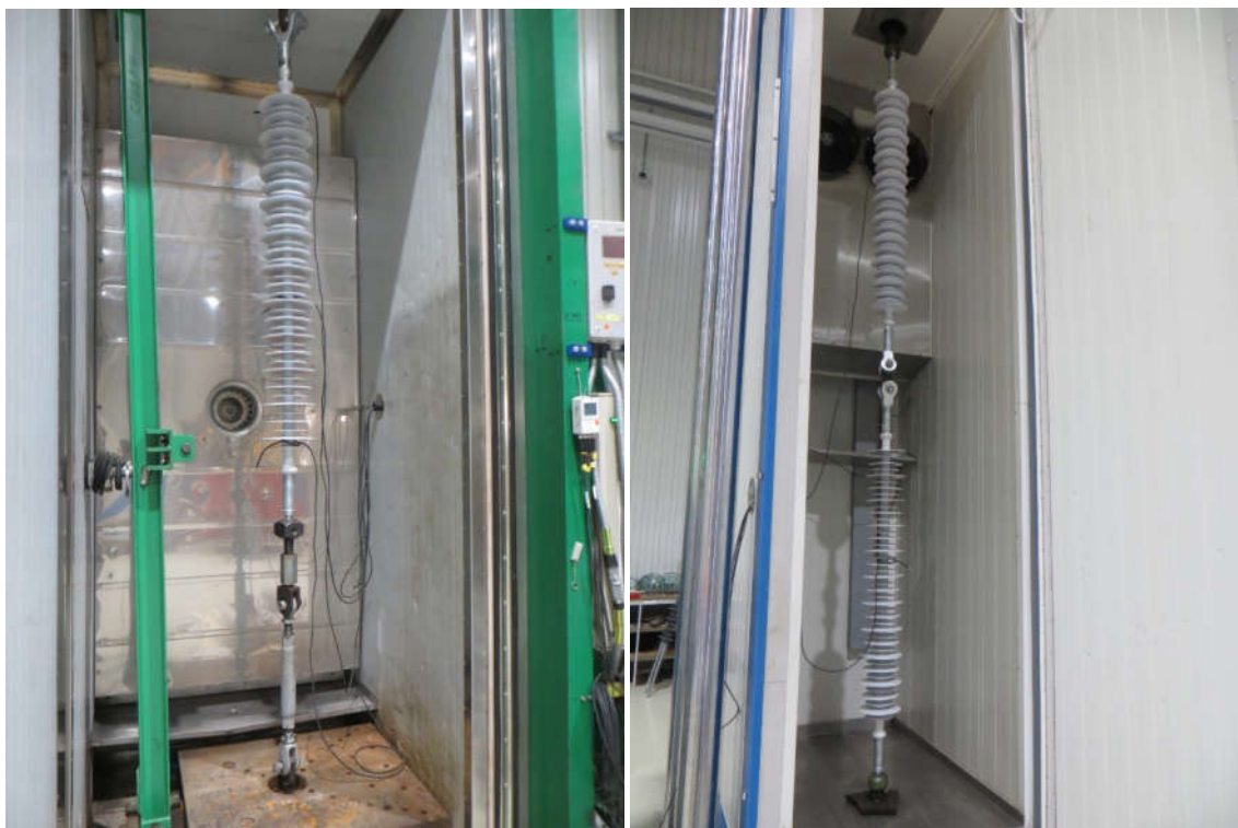
Figure 6 Test samples No. 1, 2 and 3, during thermal – mechanical test
