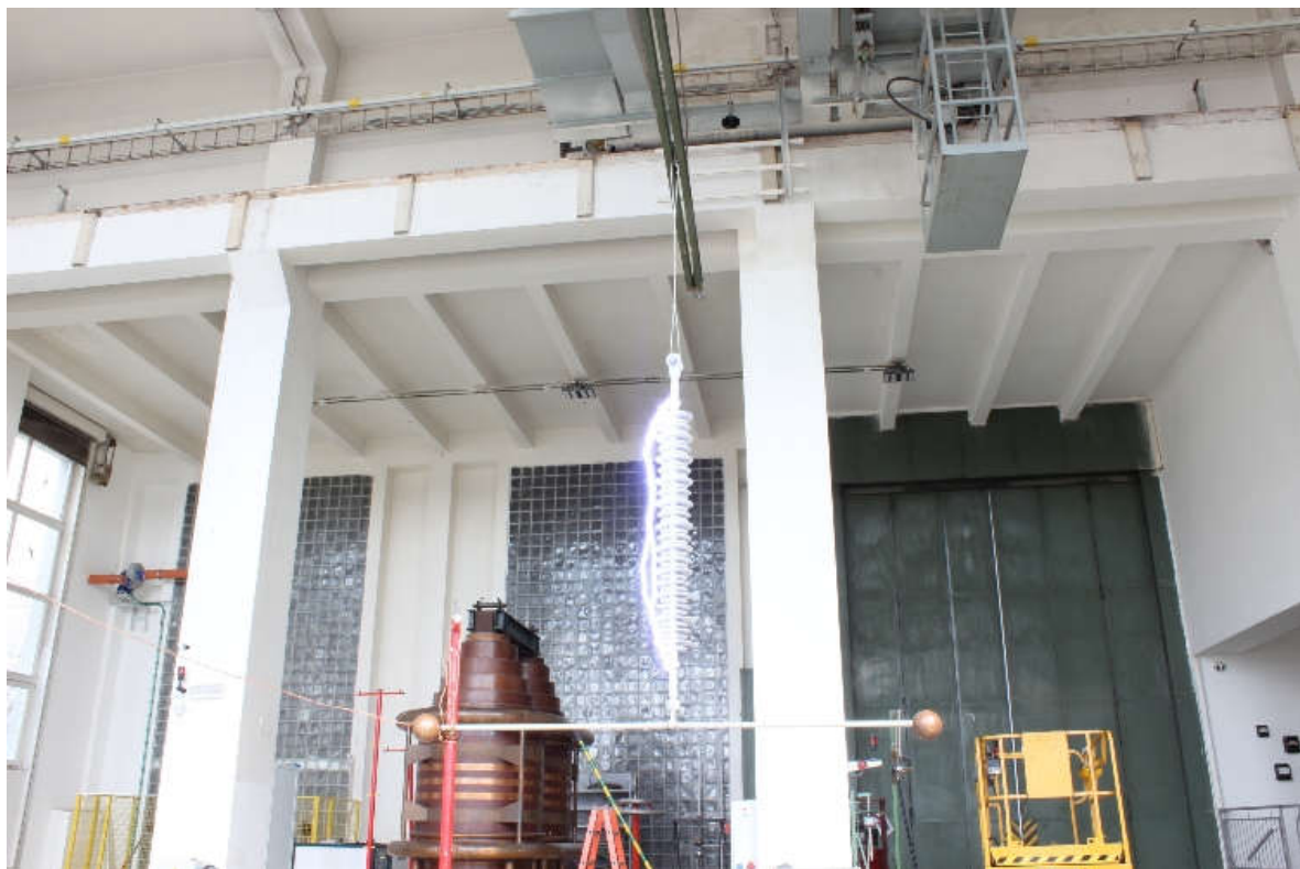
Figure 9 Test sample, during the low-frequency dry flashover voltage test
