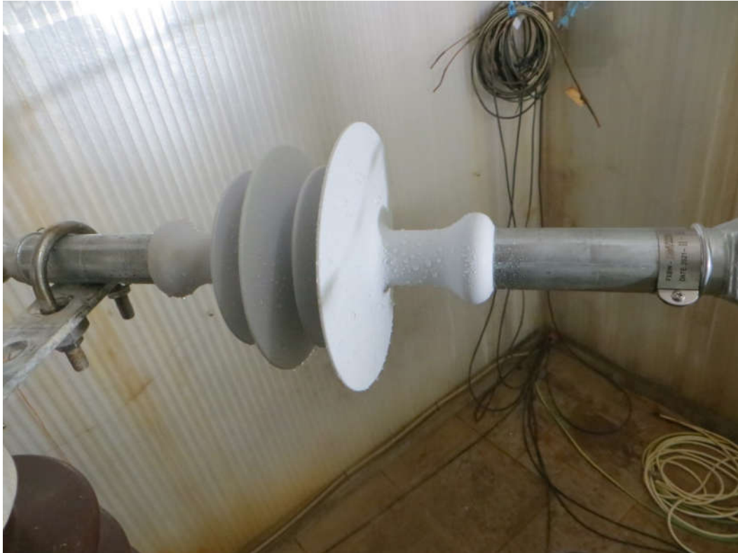
Figure 18 Test sample No. 2, horizontal position, housing tracking and erosion test
