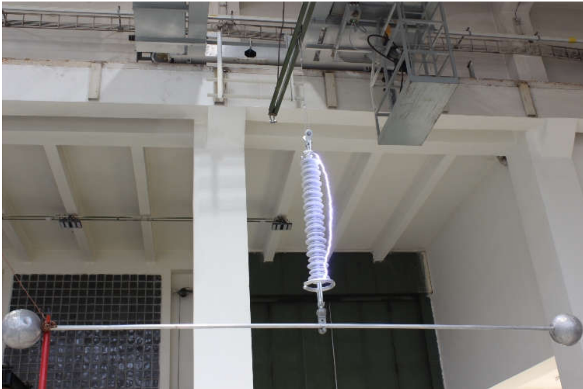
Figure 4 Test arrangement and flashover under the critical impulse flashover test
