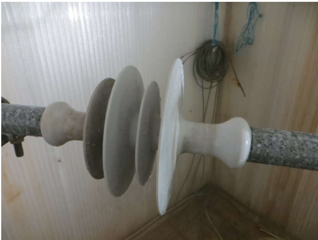
Figure 19 Test sample No. 2, horizontal position, after the housing tracking and erosion test
