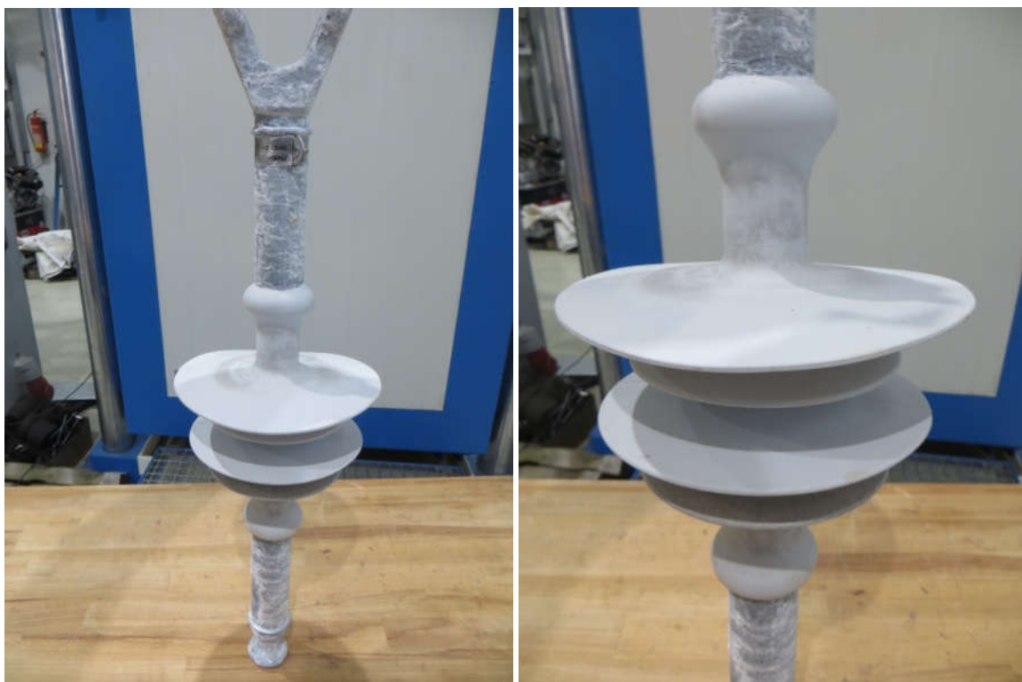
Figure 22 Test sample No. 2, horizontal sample after the housing tracking and erosion test
