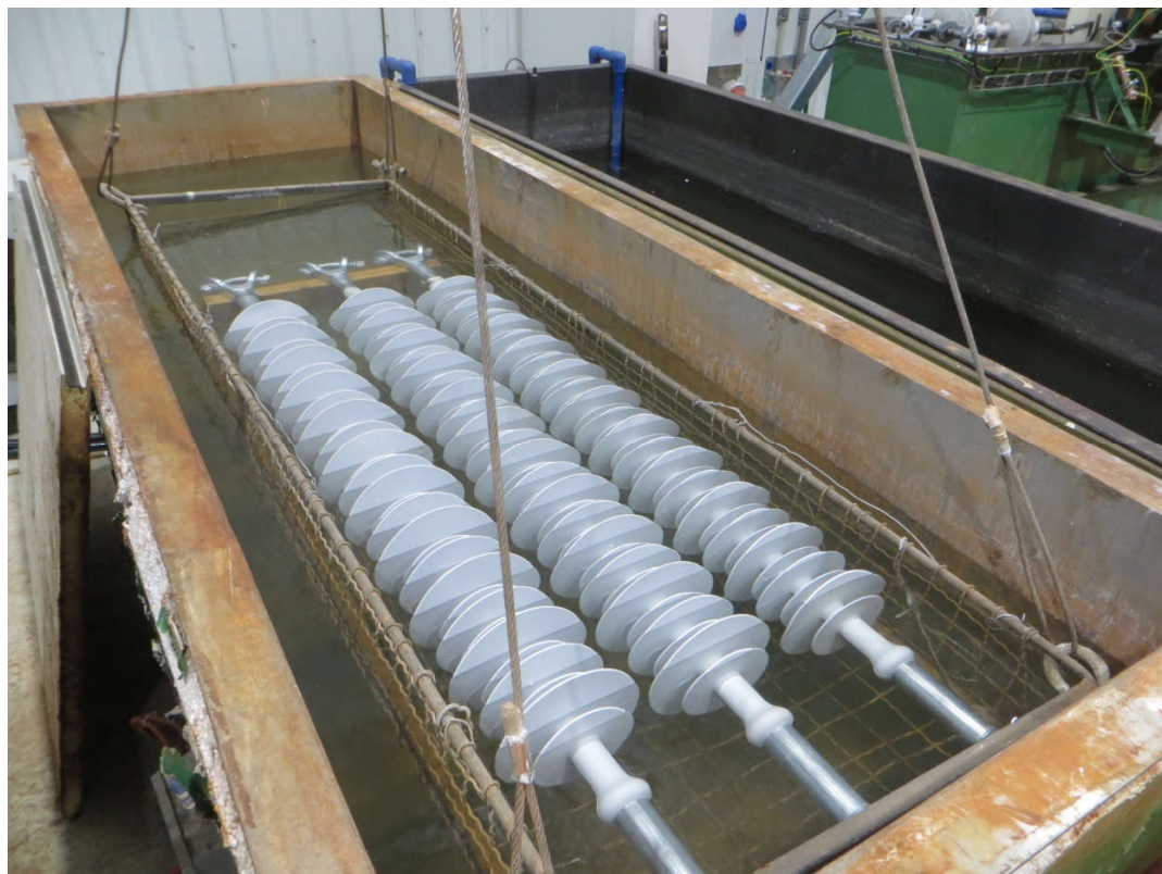
Figure 7 Test samples No. 1, 2 and 3, before water penetration test
