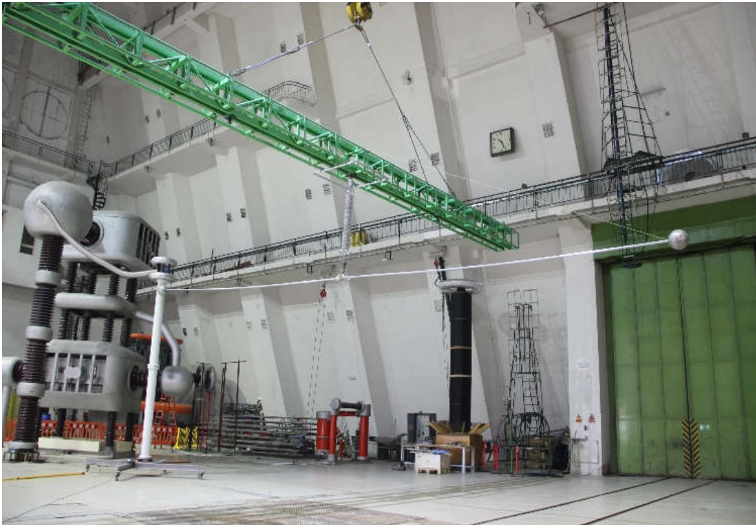
Figure 2 Test arrangement for RIV and corona tests
