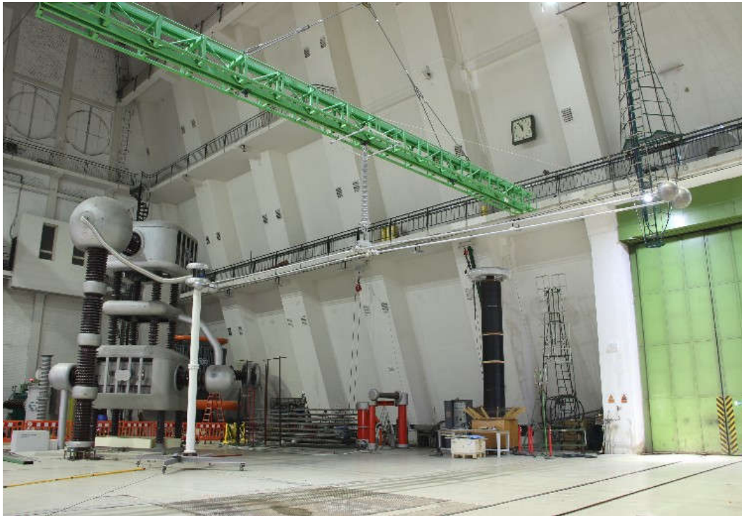
Figure 2 Test arrangement for RIV and corona tests
