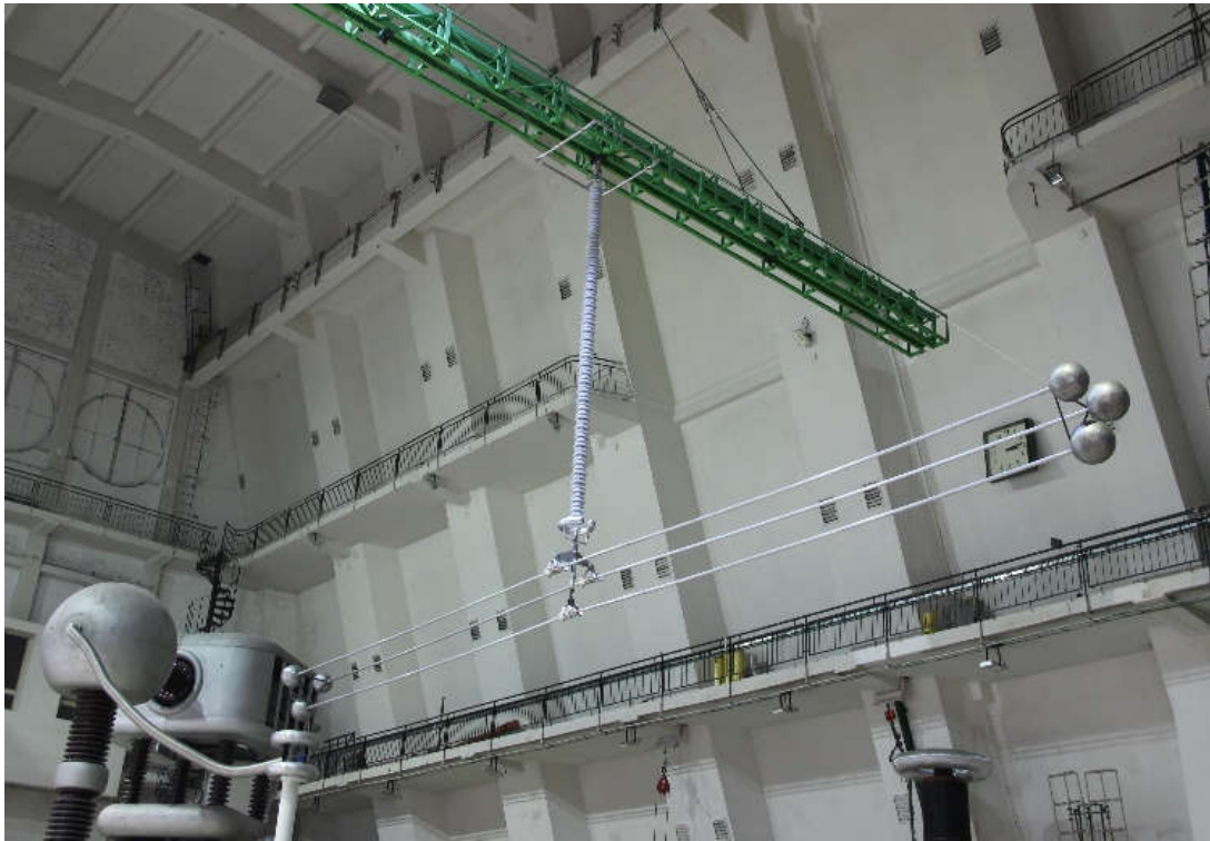
Figure 2 Test arrangement for RIV and corona tests
