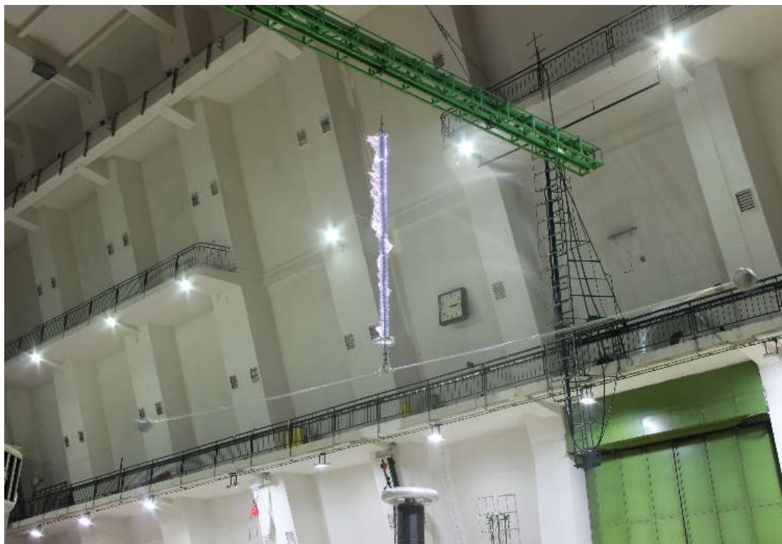
Figure 5 Test arrangement and flashover under the low-frequency wet flashover test
