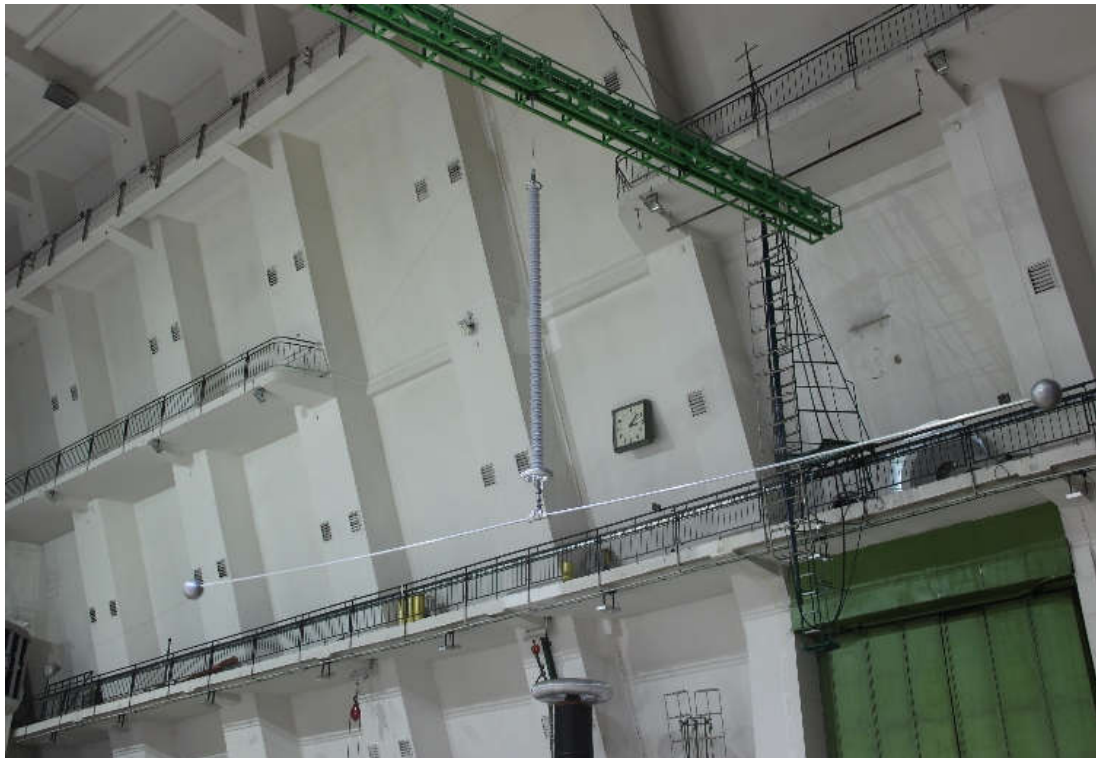
Figure 6 Test arrangement under the low-frequency dry withstand test
