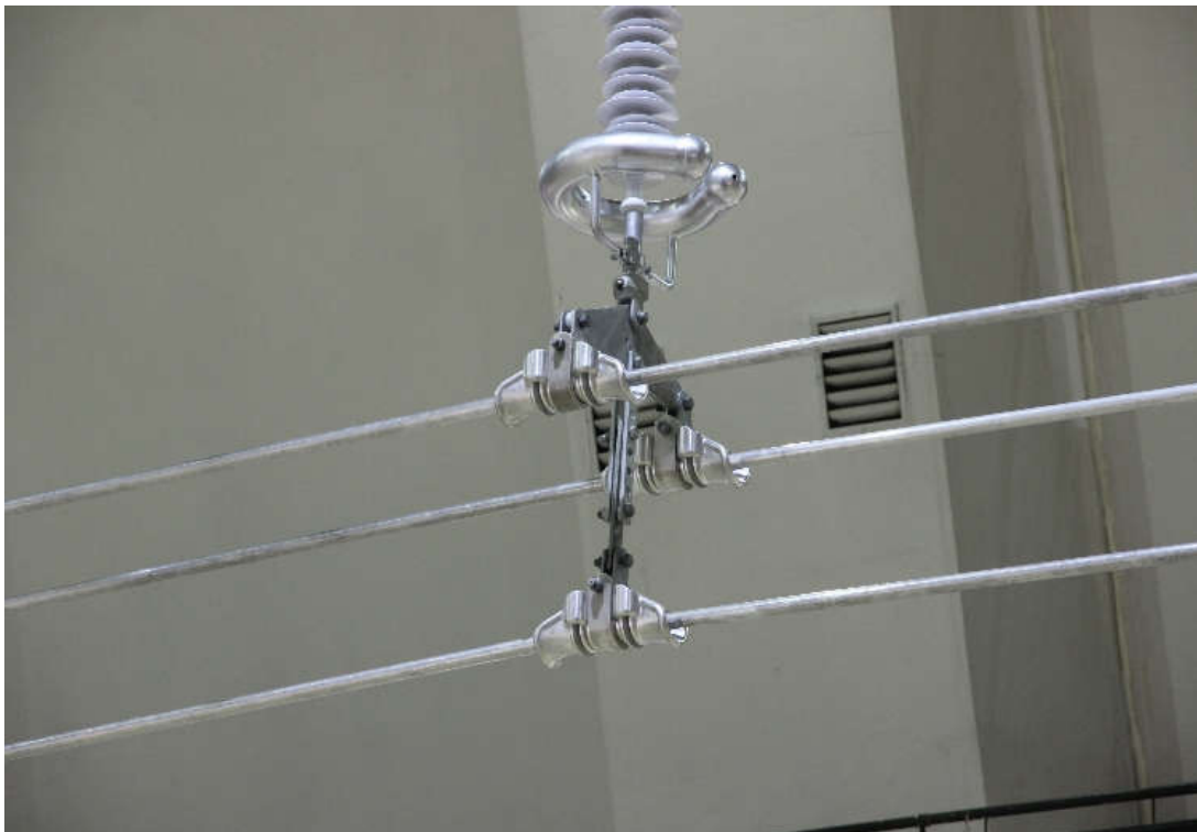
Figure 3 Test arrangement for RIV and corona tests
