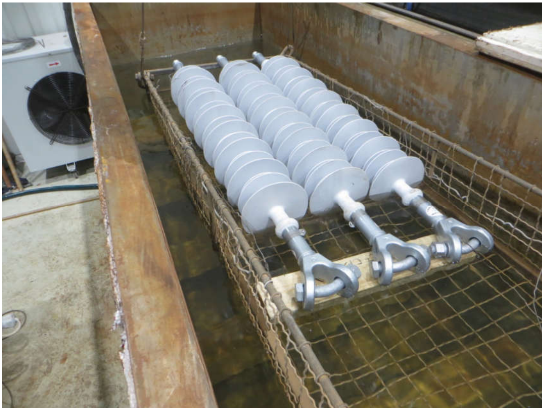
Figure 3 Test samples No. 1, 2 and 3, before watter penetration test
