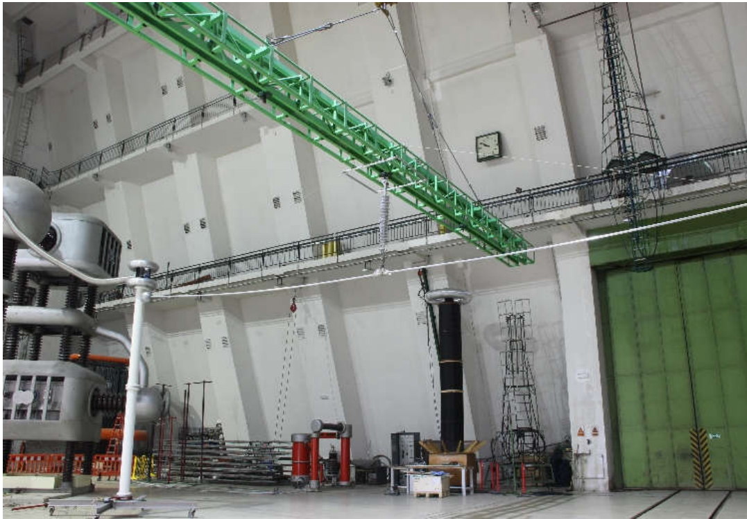
Figure 2 Test arrangement for RIV and corona tests
