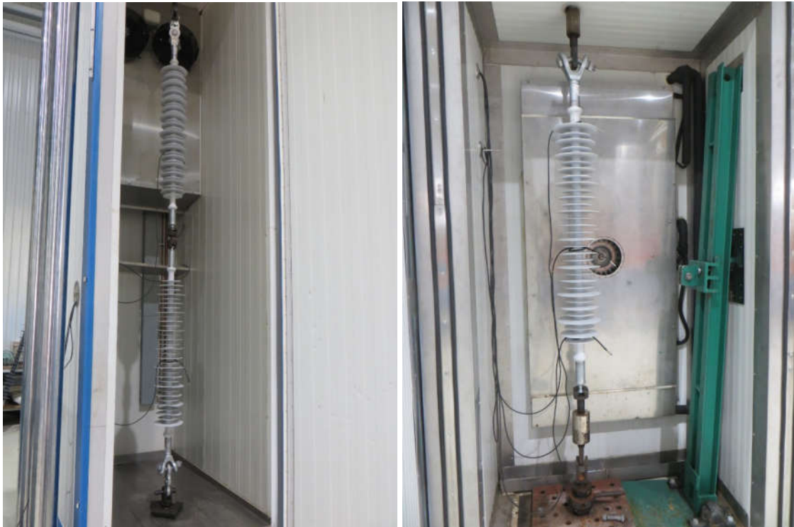
Figure 2 Test samples No. 1, 2 and 3, during thermal – mechanical test
