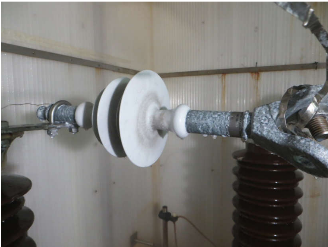
Figure 15 Test sample No. 2, horizontal position, after the housing tracking and erosion test
