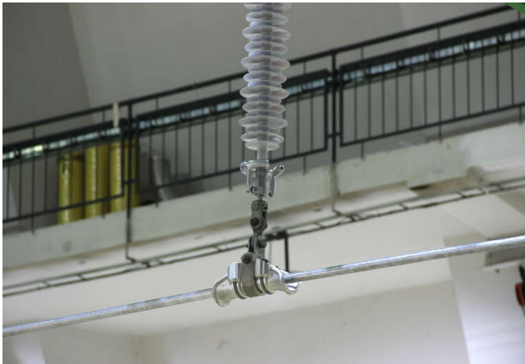
Figure 3 Test arrangement for RIV and corona tests
