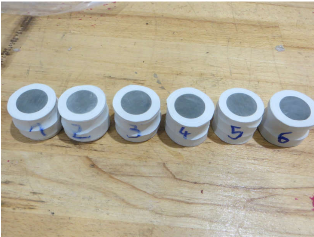
Figure 13 Test specimens after the voltage test – water diffusion test
