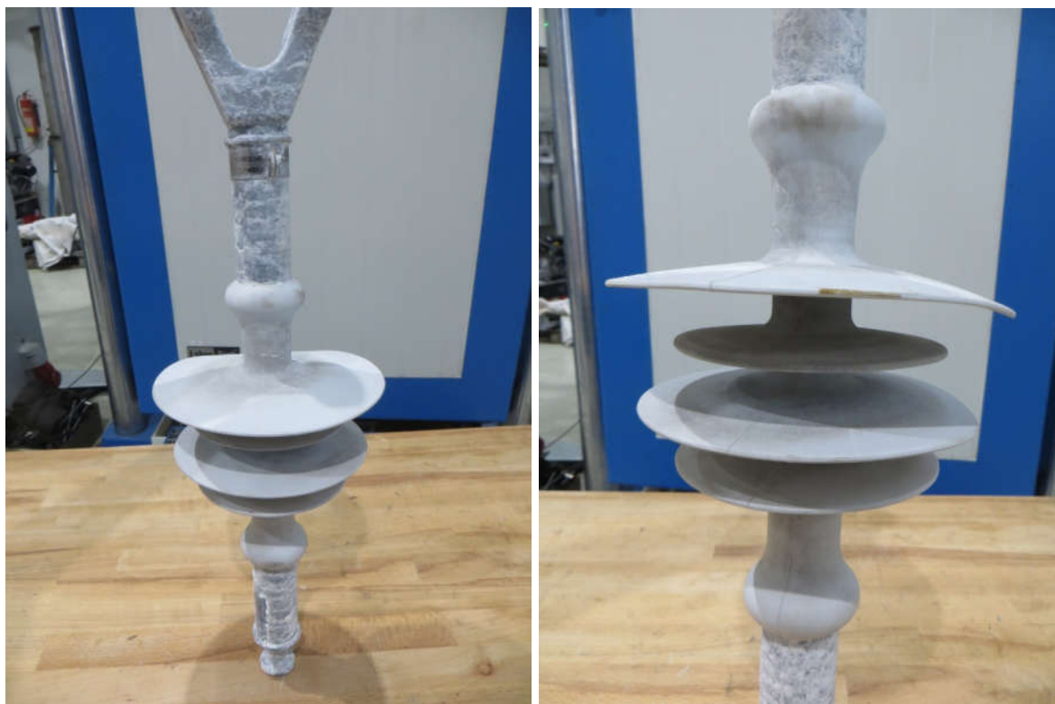
Figure 18 Test sample No. 1, vertical sample after the housing tracking and erosion test
