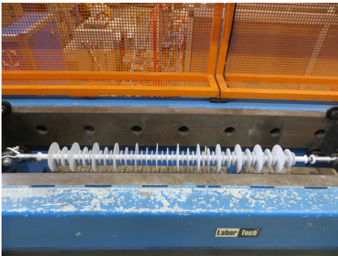
Figure 43 Mechanical load-time test, failing load test, test sample No. 26
