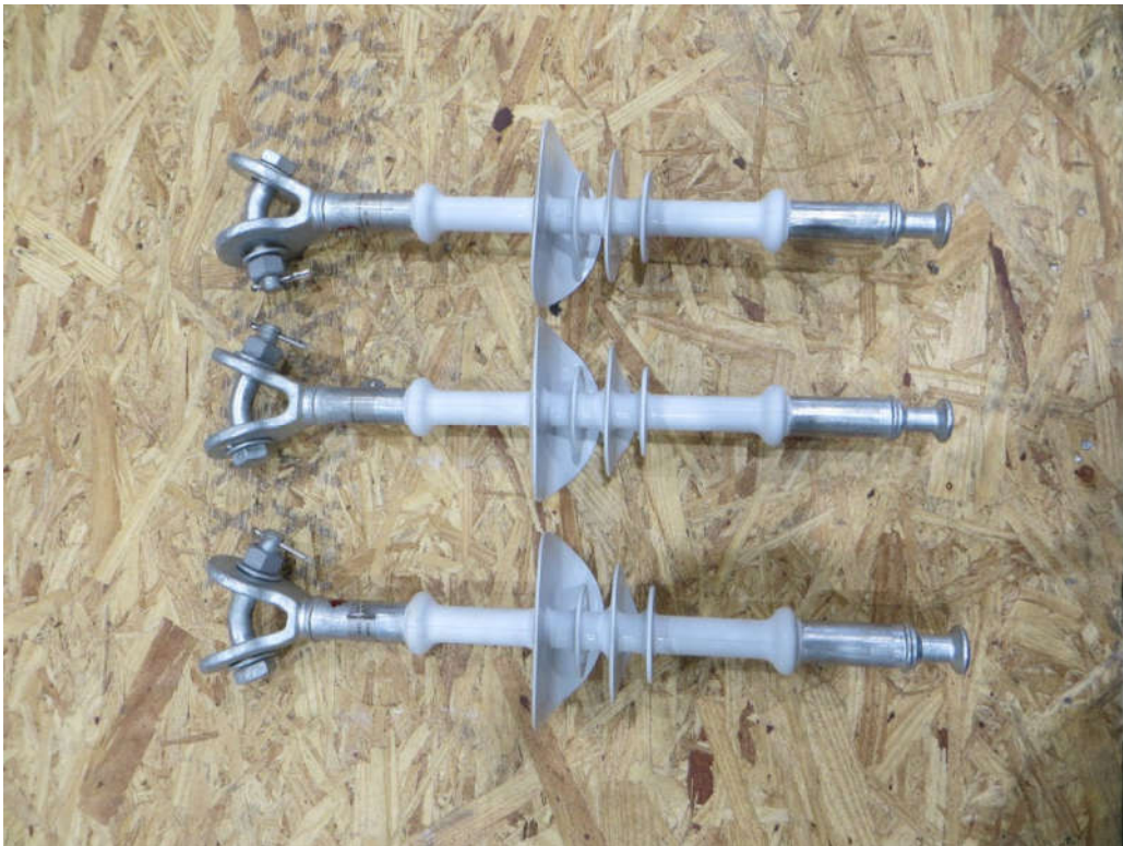
Figure 4 Composite line insulator test samples No. 1, 2 and 3 before tracking and erosion test
