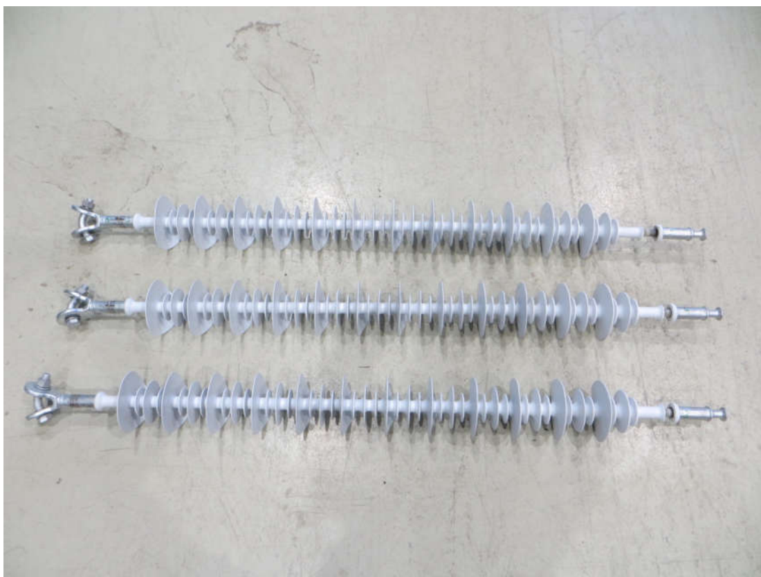
Figure 27 Test samples No. 3, 4 and 5, after tensile load test
