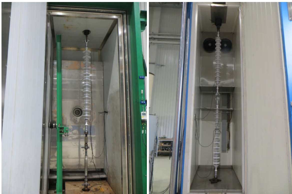
Figure 28 Test samples No. 23, 24 and 25 during thermal mechanical test
