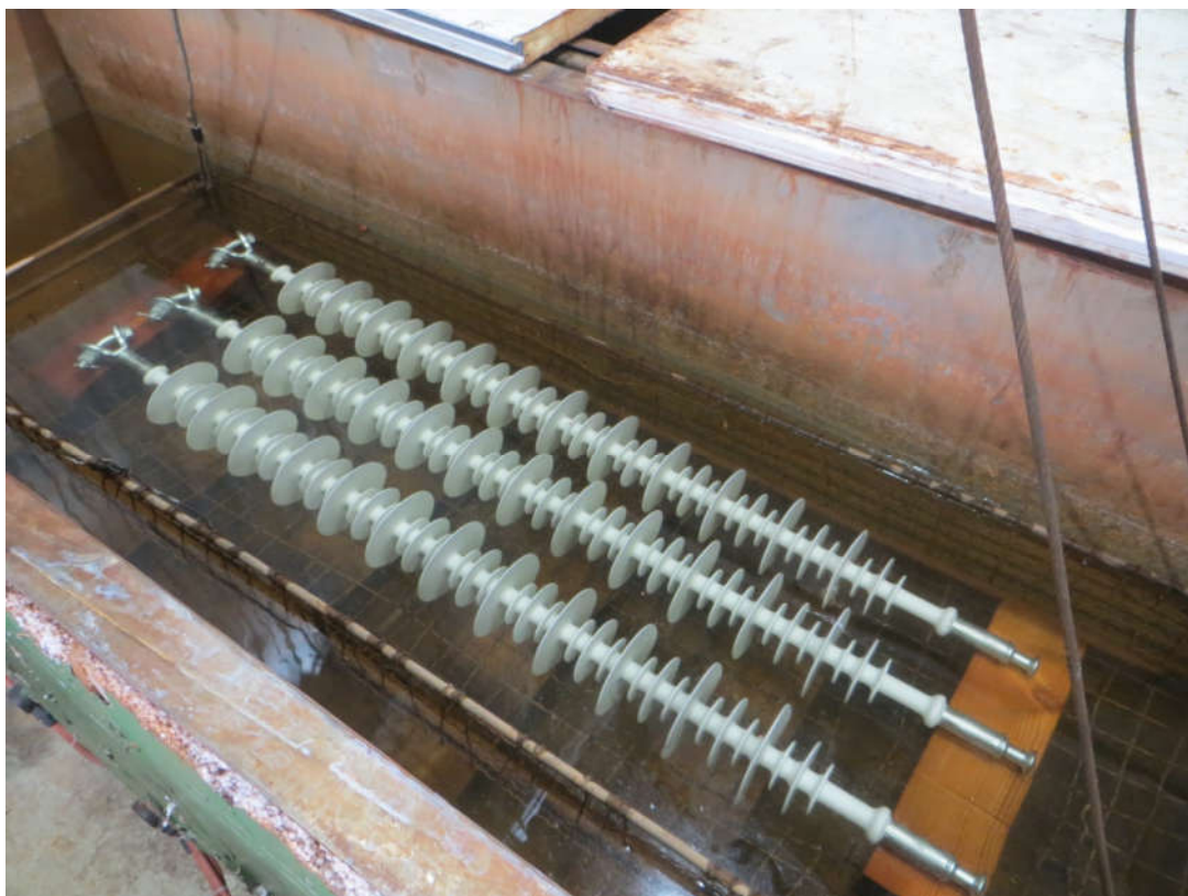
Figure 21 Boiling of the test samples (water penetration test)
