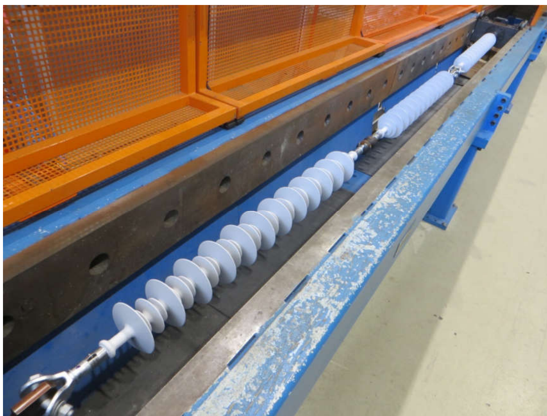
Figure 39 Assembled core load-time test, withstand tensile load test, test samples No. 9, 10 and 11
