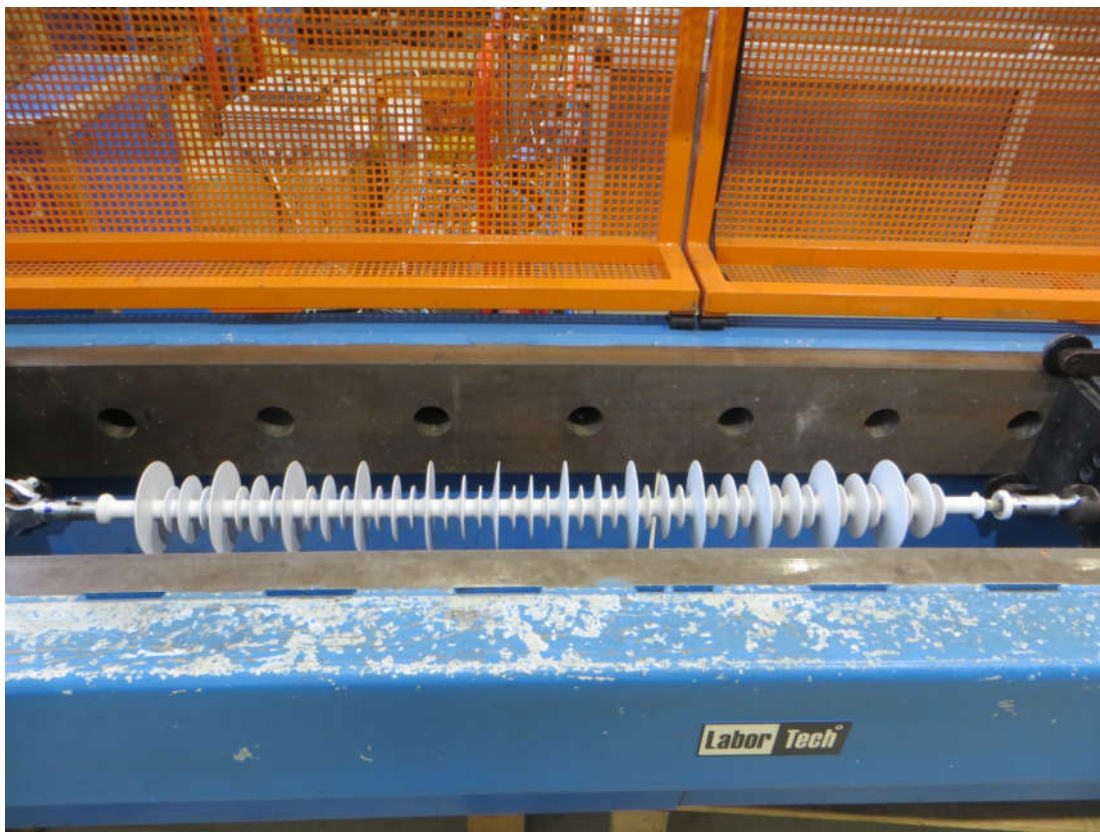
Figure 35 Assembled core load-time test, test sample No. 7
