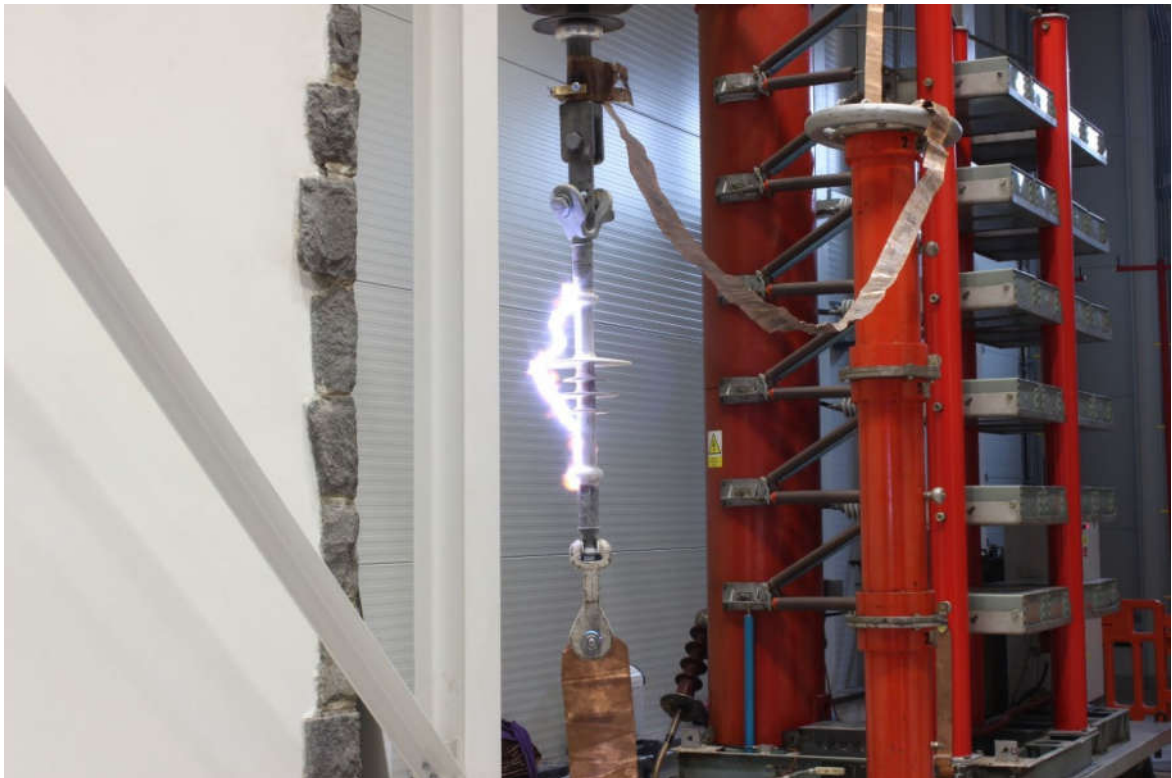
Figure 8 Composite line insulator during the steep front impulse voltage test
