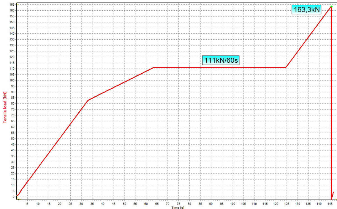
Figure 16 Record of mechanical failing test, test sample No. 27 (mechanical load-time test)
