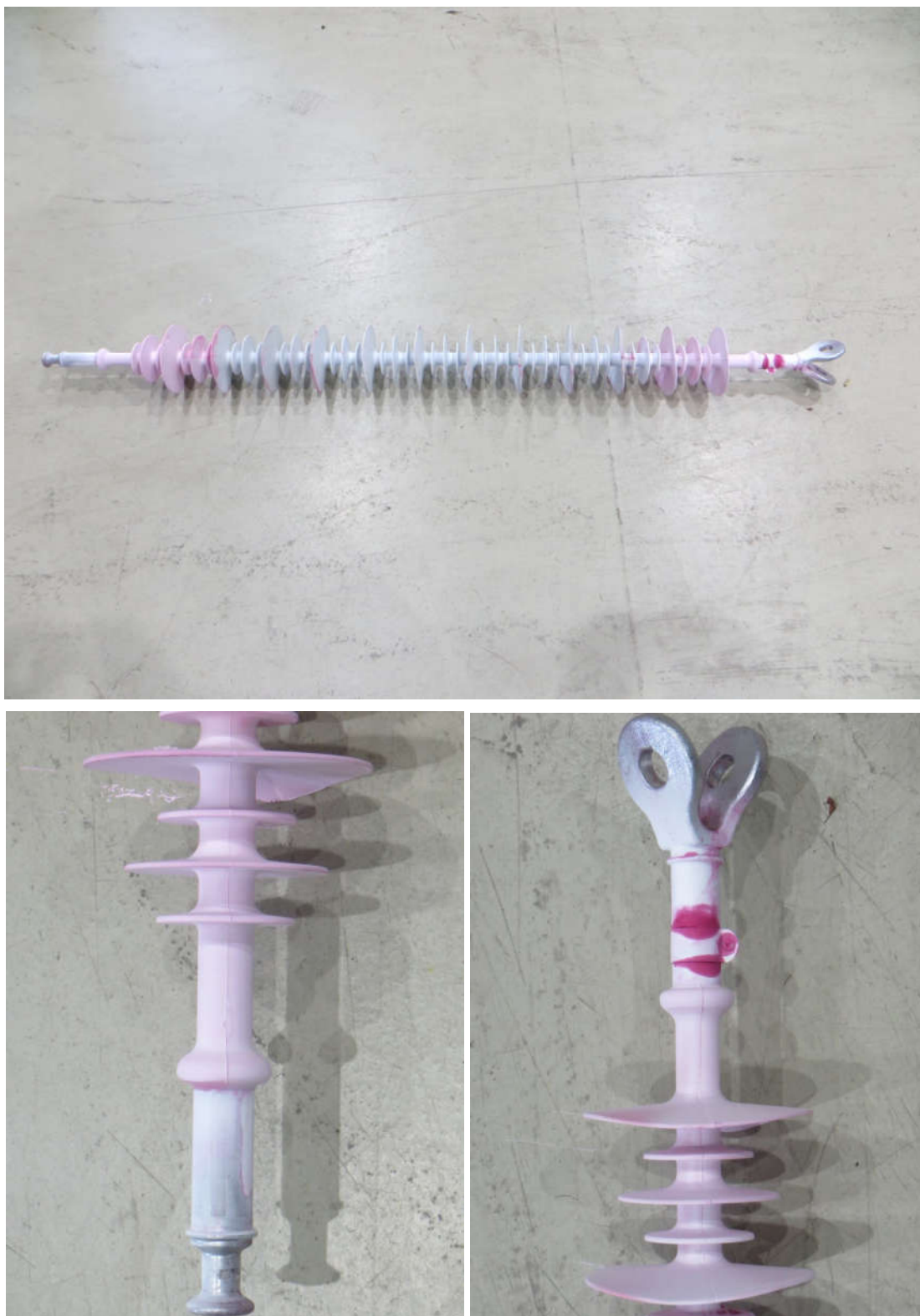
Figure 47 Mechanical load-time test, test samples No. 29 after dye penetration test
