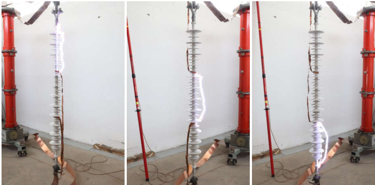
Figure 22 Test sample during steep-front impulse voltage test (water penetration test)
