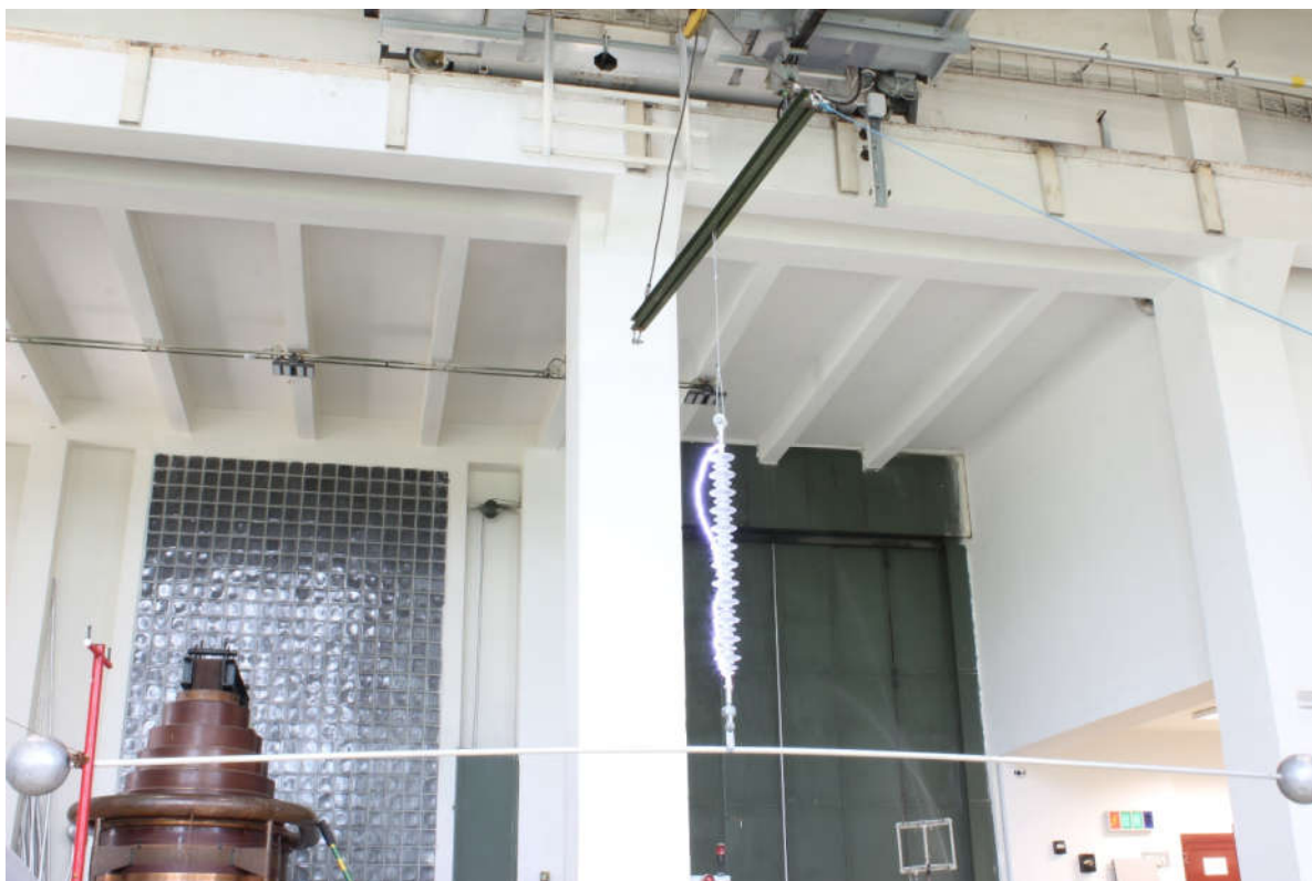
Figure 7 Test arrangement and flashover under the wet power frequency voltage flashover test
