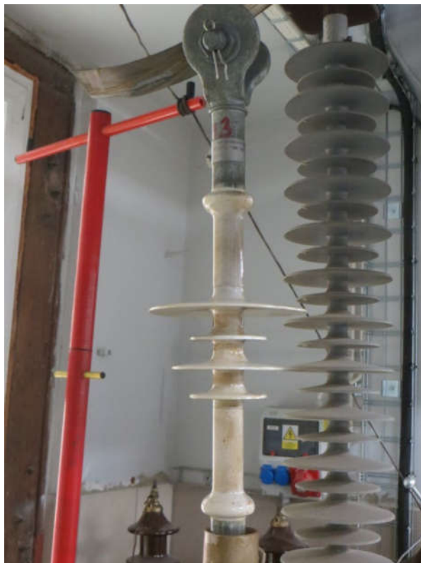
Figure 6 Composite line insulator, test sample No.3, after tracking and erosion test
