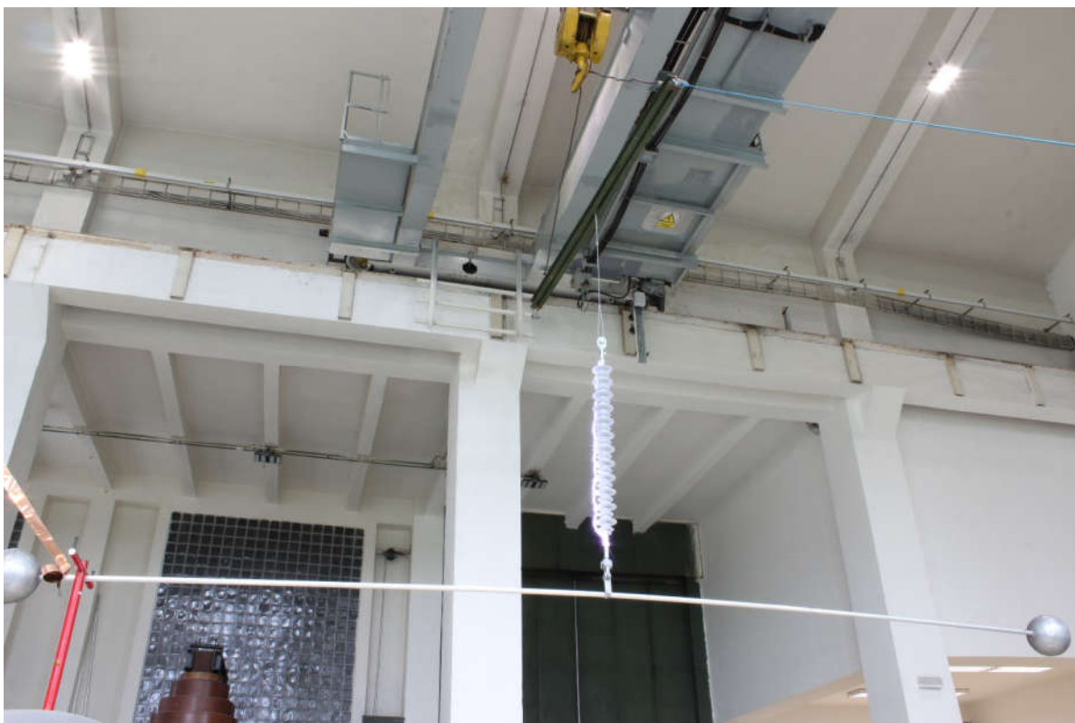
Figure 6 Test arrangement and flashover under the critical impulse flashover test
