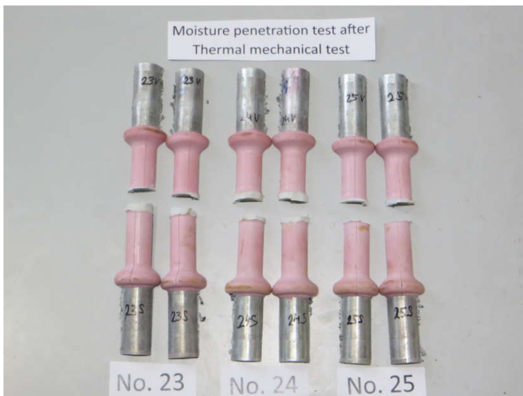
Figure 30 Test samples after cut of end metal fittings (moisture penetration test after thermal mechanical test)
