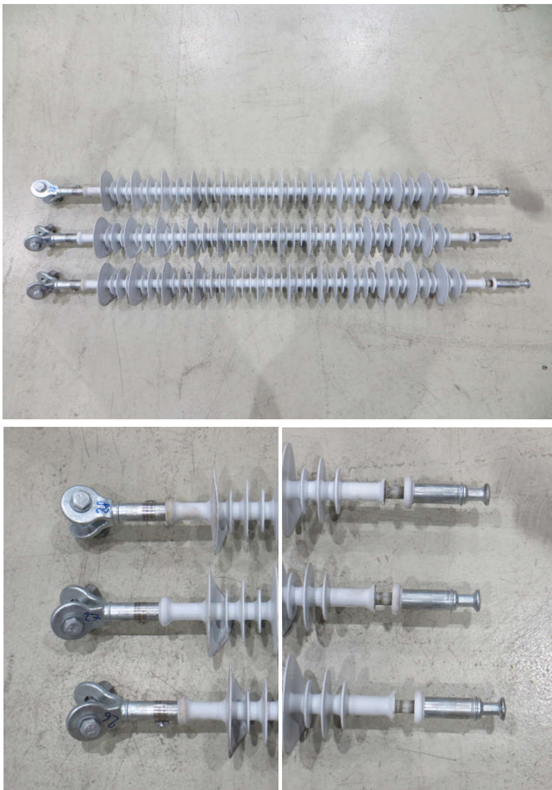
Figure 46 Mechanical load-time test, test samples No. 26, 27 and 28 after mechanical failing load test
