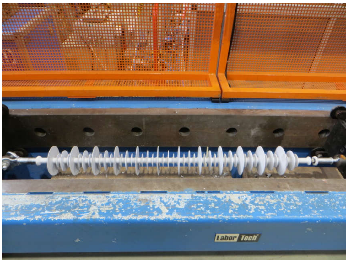
Figure 44 Mechanical load-time test, failing load test, test sample No. 27
