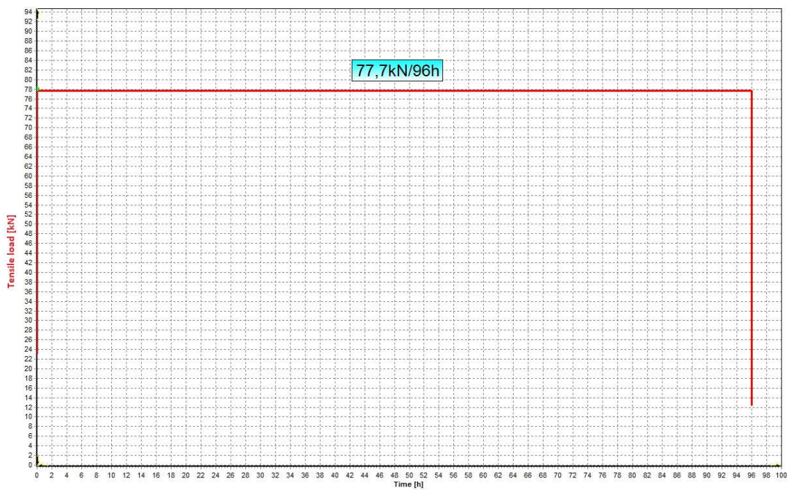
Figure 14 Record of mechanical withstand load test, test samples No. 26, 27, 28 and 29 (mechanical load-time test)
