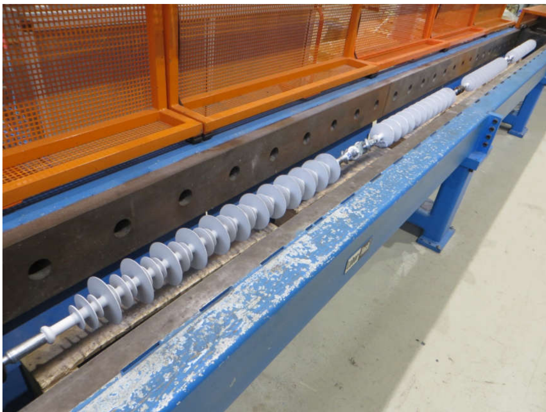
Figure 42 Mechanical load-time test, withstand tensile load test, test samples No. 26, 27, 28 and 29
