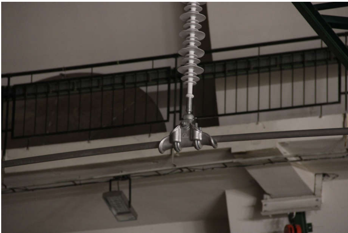
Figure 5 Test arrangement under corona test at 100 kV (no visible corona)
